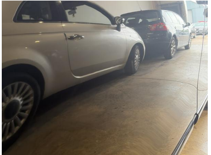
16: Door osr Dented Over 30mm
