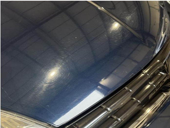
1: Bonnet Scratched Over 25mm Thru Paint
