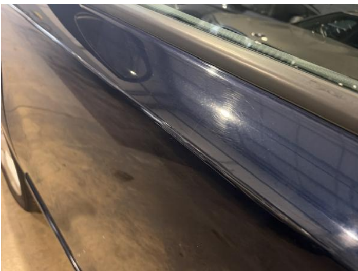
7: Door nsf Dented Between 10mm + 30mm
