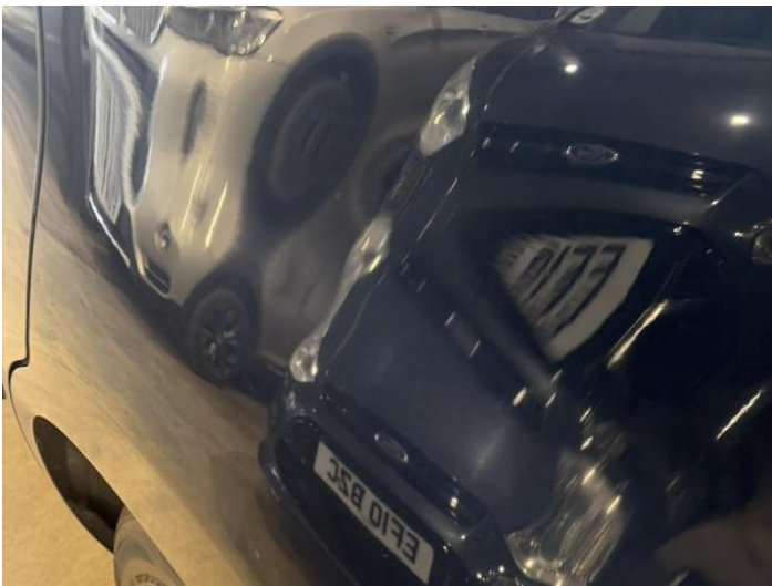
11: Qtr Panel nsr Scratched UpTo 25mm Thru Paint
