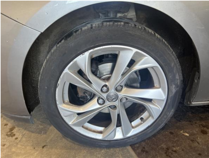
15: Wheel nsf Scratched Over 50mm
