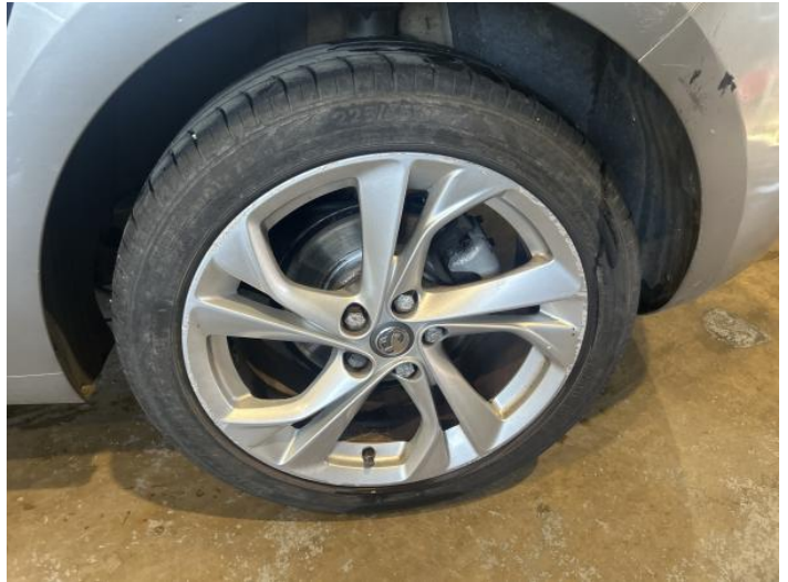
10: Wheel nsr Scratched Over 50mm
