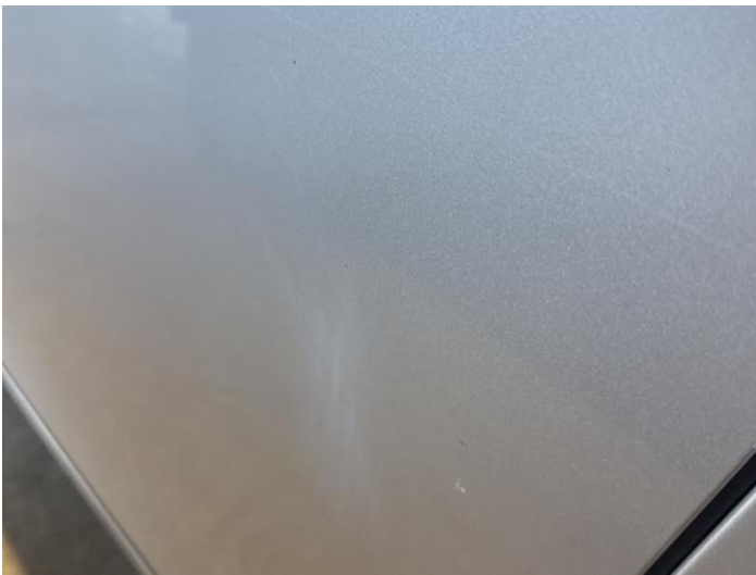
5: Door nsf Scratched Over 25mm Thru Paint
