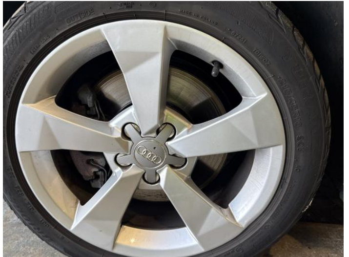
4: Wheel nsf Dented UpTo 30mm (Alloy)
