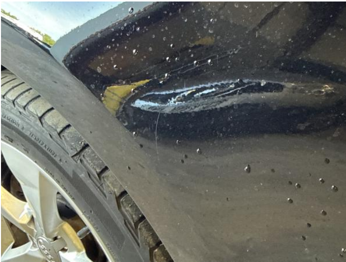
5: Wing nsf Scratched Over 25mm Thru Paint
