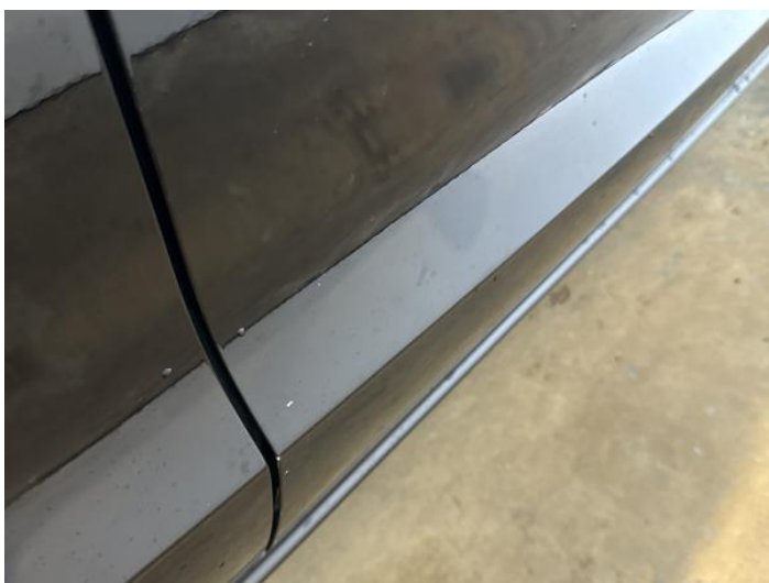
13: Door osf Chipped Edge Chip
