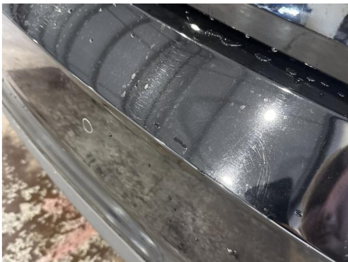
9: Bumper Rear Scratched 25 to 100mm Thru Paint
