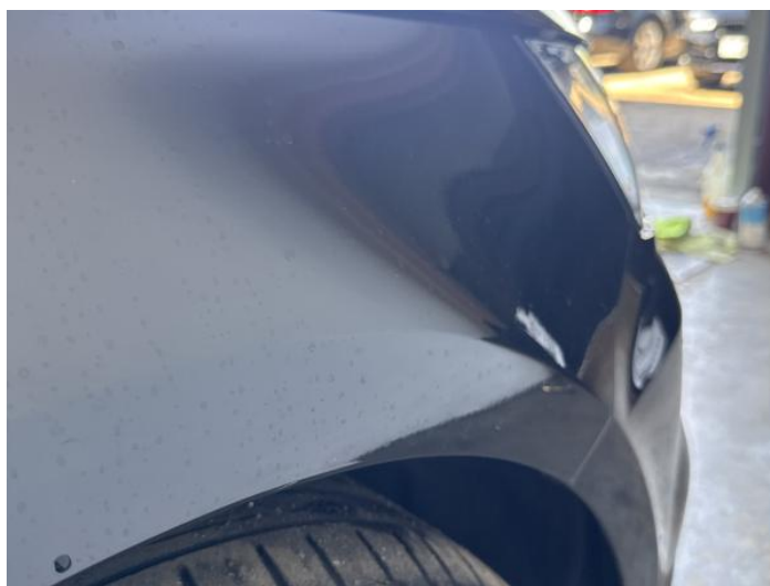
14: Wing osf Scratched UpTo 25mm Thru Paint
