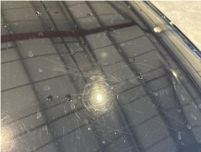
3: Bonnet Scratched Over 25mm Thru Paint
