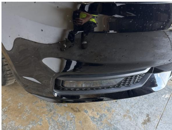
2: Bumper Front Scratched 25 to 100mm Thru Paint
