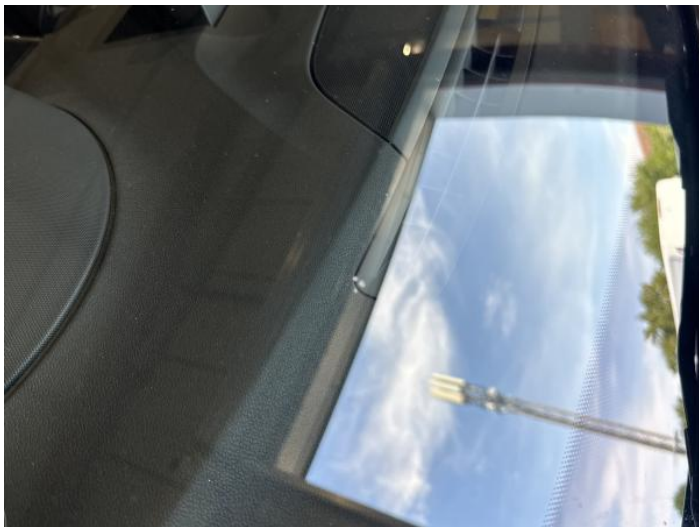
15: Screen Front Chipped UpTo 10mm
