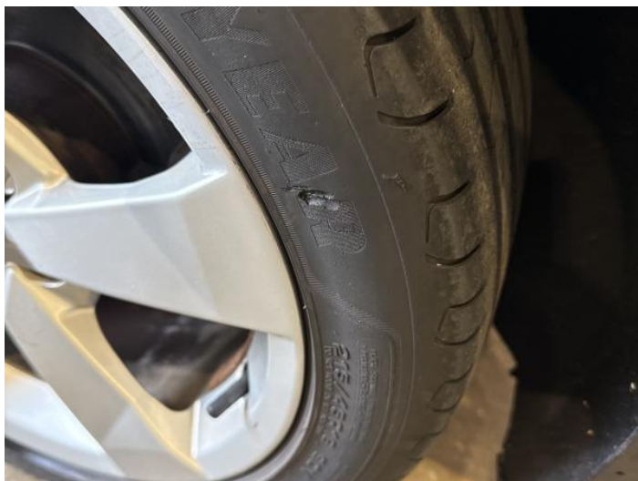
1: Tyre nsr Damaged Replace
