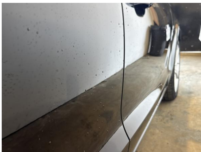
12: Door osr Dented Between 10mm + 30mm
