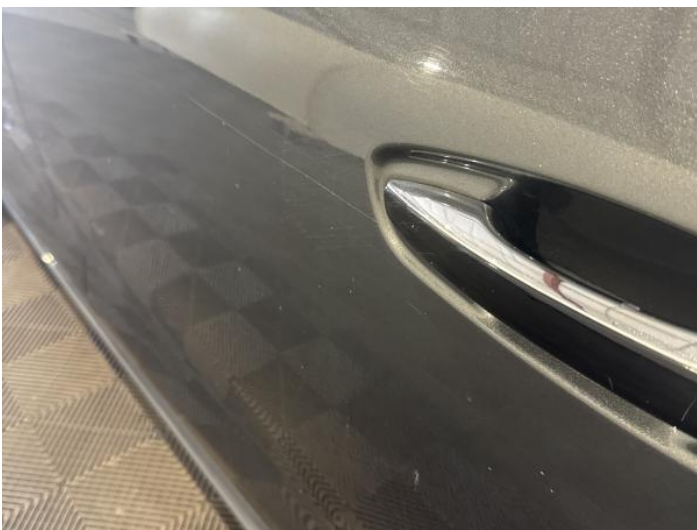
7: Door nsr Scratched Over 25mm Thru Paint
