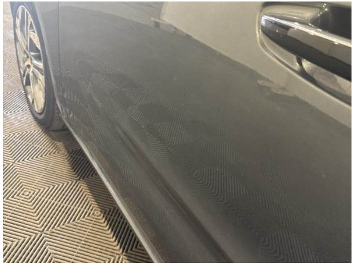
6: Door nsf Chipped Multiple Chips
