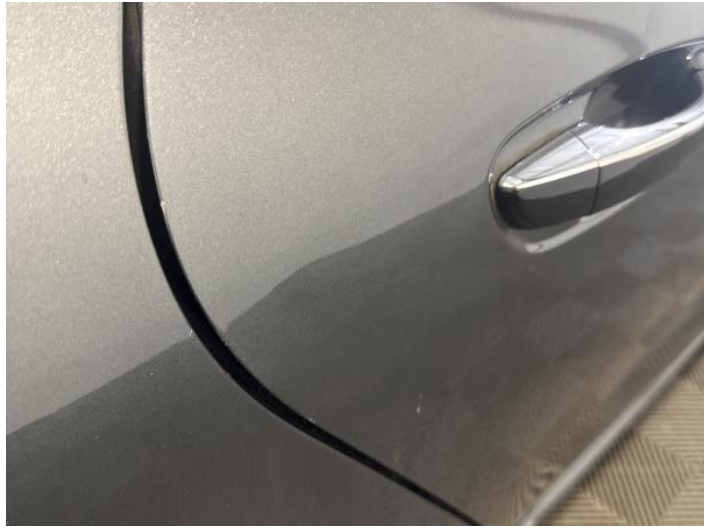
16: Door osr Dented Between 10mm + 30mm
