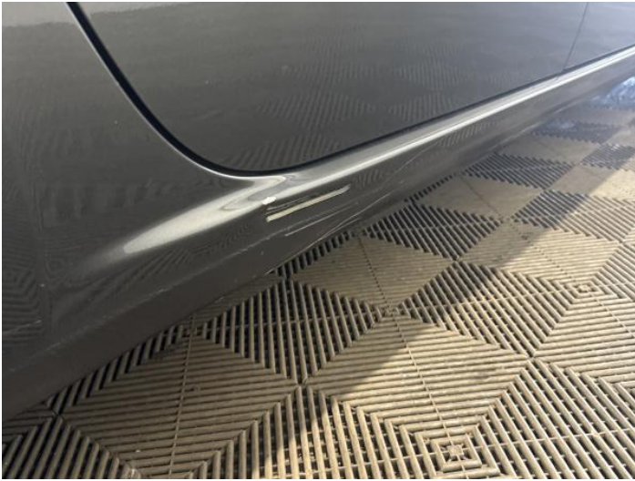
15: Sill os Dented With Paint Damage
