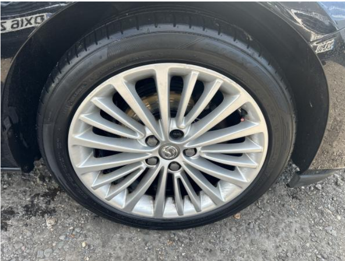
1: Wheel osf Scratched Over 50mm
