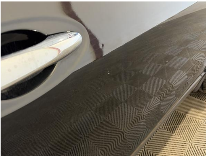
17: Door osf Scratched UpTo 25mm Thru Paint
