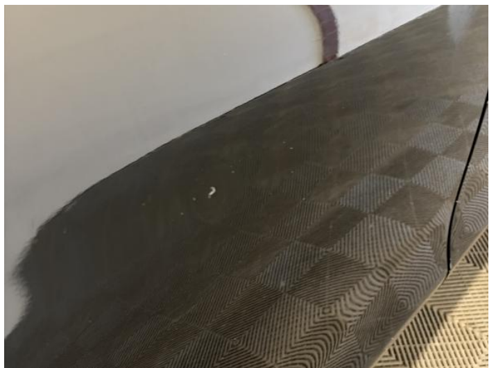
14: Door osr Dented Between 10mm + 30mm
