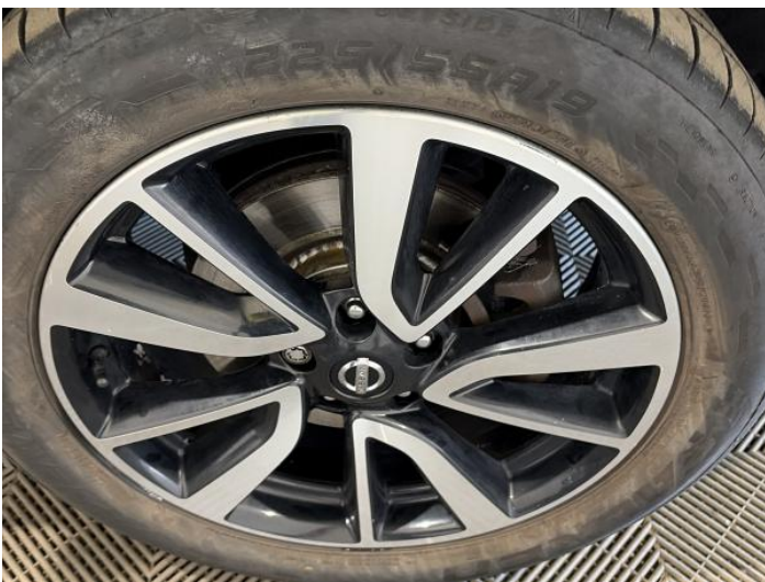
19: Wheel osf Scratched Over 50mm
