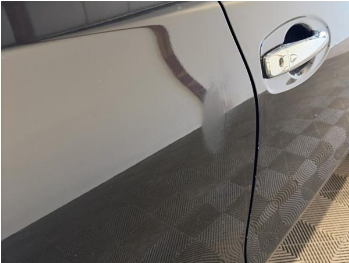
15: Door osr Scratched Over 25mm Thru Paint
