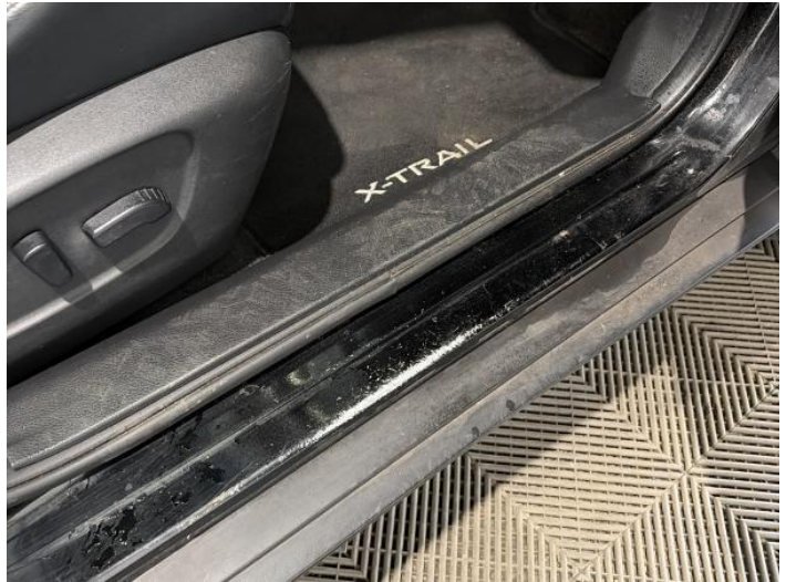
22: Sill os Scratched Over 25mm Thru Paint
