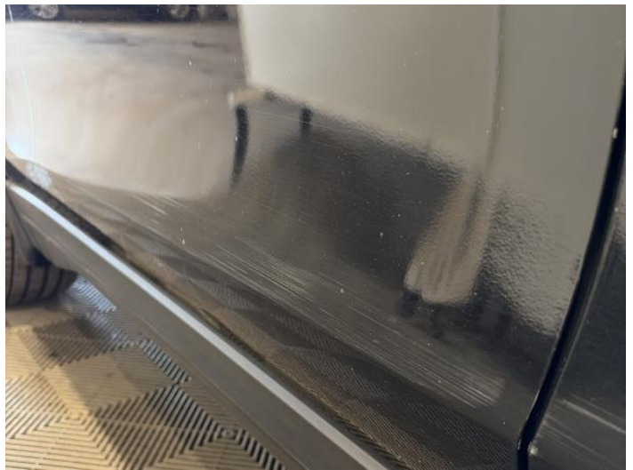
6: Door nsf Scratched Over 25mm Thru Paint
