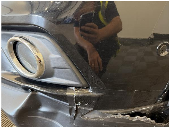
2: Bumper Front Cracked UpTo 25mm
