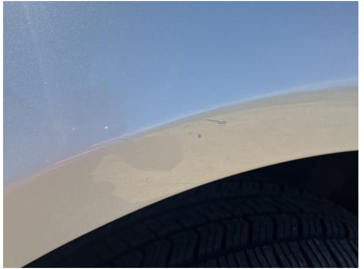
4: Wing nsf Scratched Over 25mm Thru Paint
