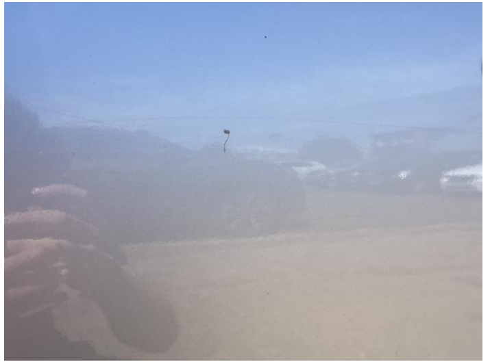
6: Door nsf Scratched Over 25mm Thru Paint
