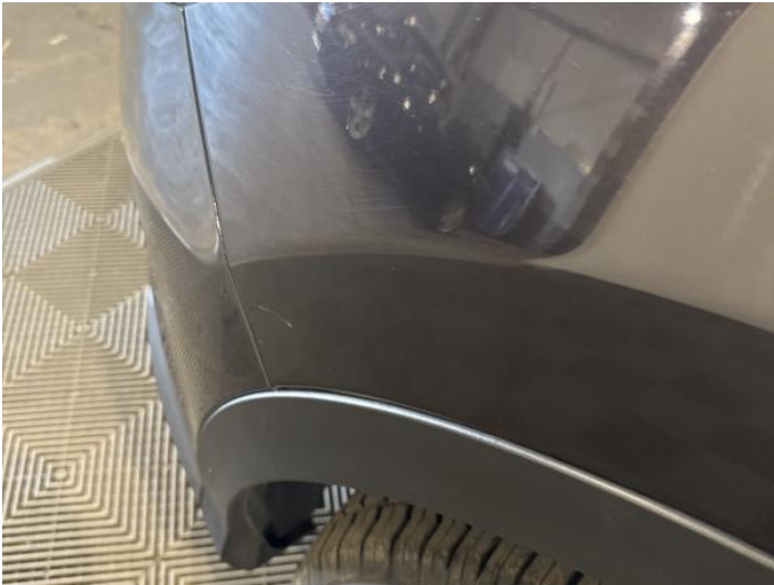
3: Wing nsf Scratched Over 25mm Thru Paint
