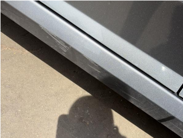
15: Sill Panel Trim ns Scratched (Painted) Over 25mm Thru Paint
