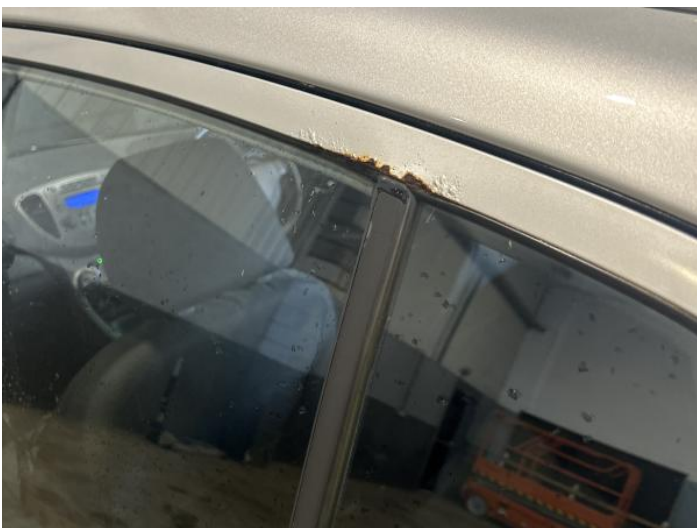
7: Door nsr Rusted Over 5mm
