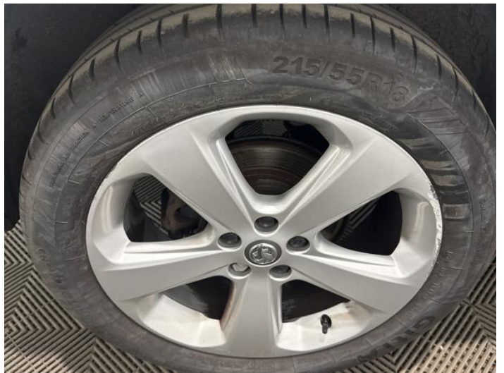
12: Wheel osr Scratched Over 50mm
