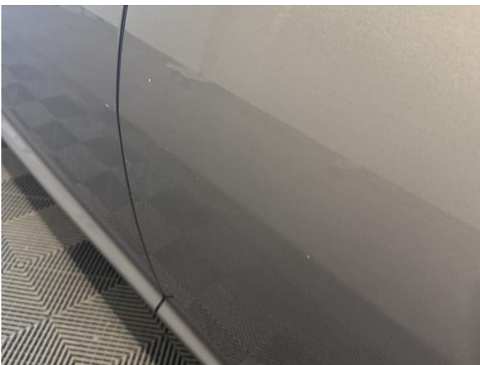
7: Door nsr Scratched Over 25mm Thru Paint
