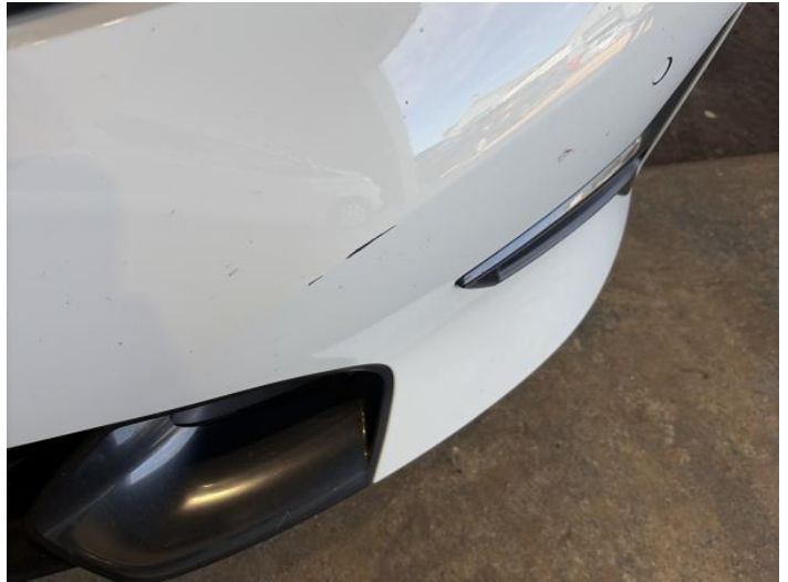
10: Bumper Front Scratched 25 to 100mm Thru Paint
