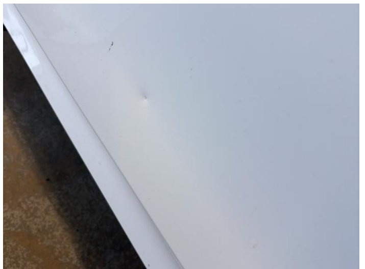
8: Door nsf Dented 2 Or Less UpTo 10mm
