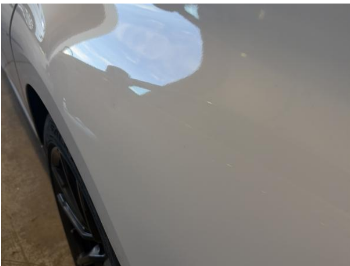
7: Qtr Panel nsr Dented Between 10mm + 30mm
