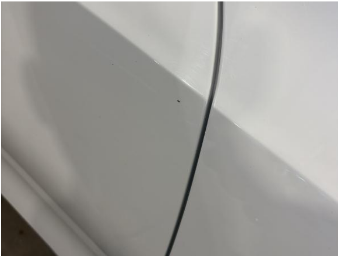
1: Door osf Chipped 1 To 5
