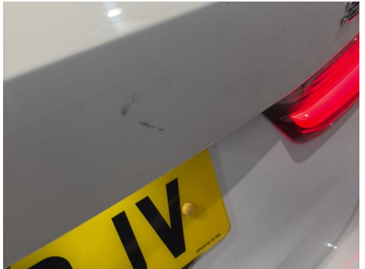
6: Tailgate Scratched Over 25mm Thru Paint
