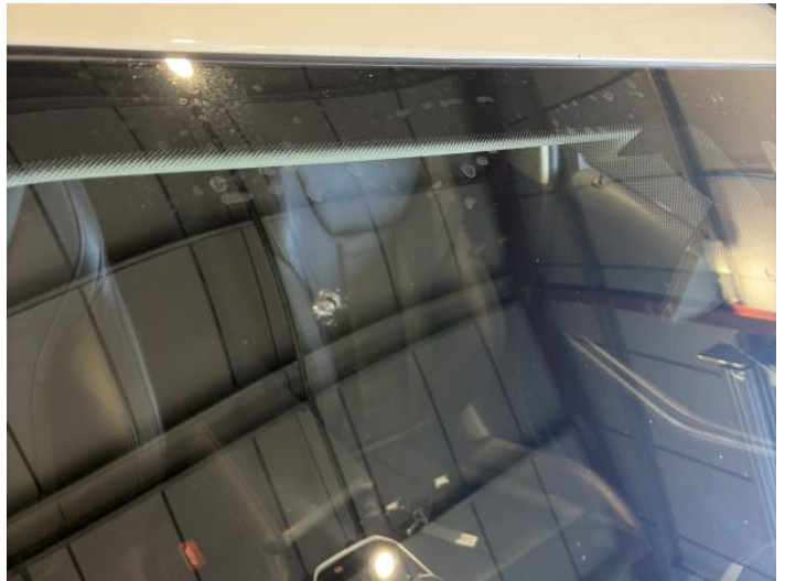
12: Screen Front Chipped Over 10mm
