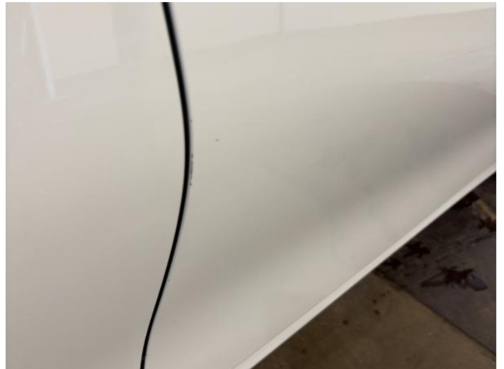
2: Door osf Chipped Edge Chip
