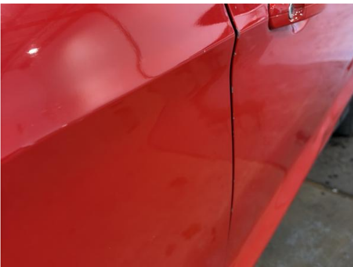
13: Door osr Dented Between 10mm + 30mm
