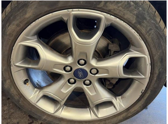
16: Wheel osf Scratched Over 50mm
