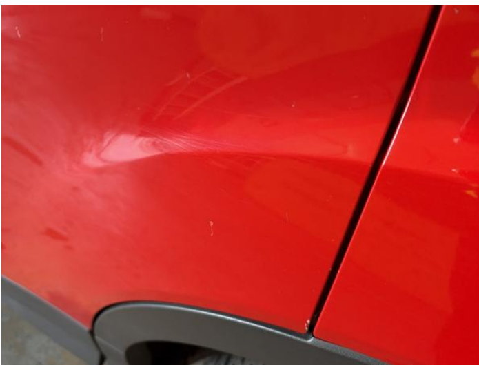
7: Door nsr Chipped Edge Chip
