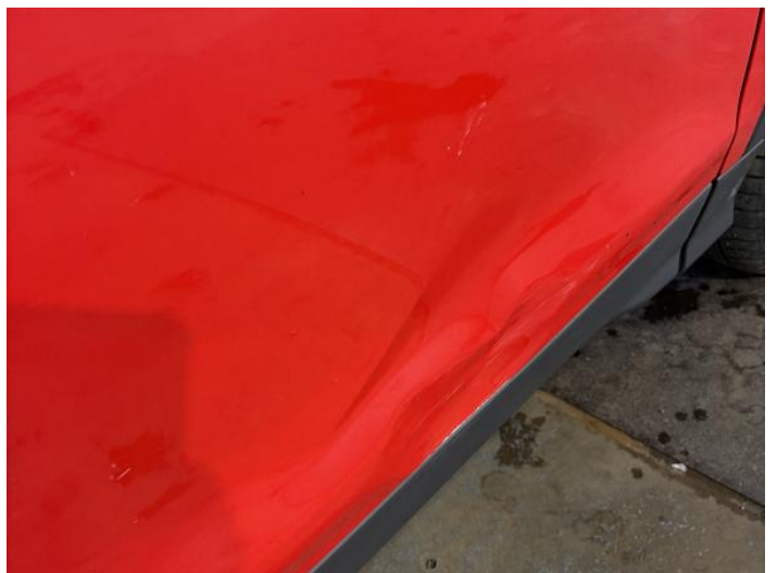
14: Door osf Dented With Paint Damage
