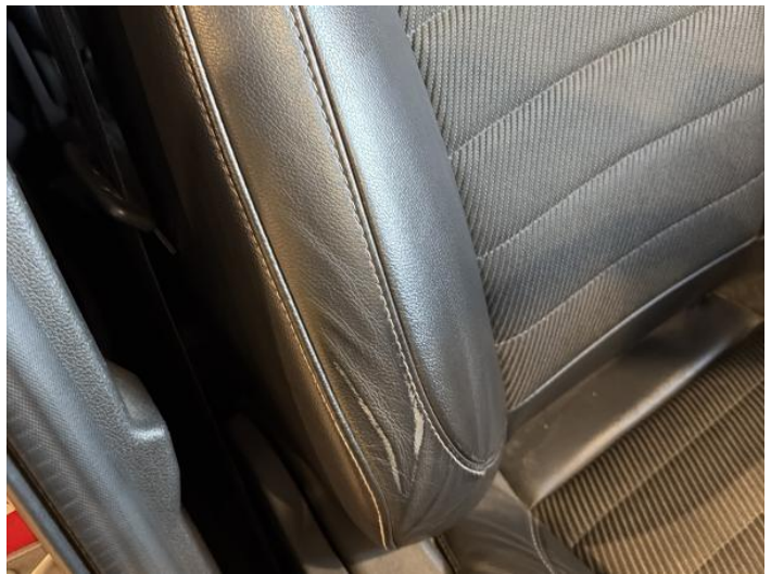
18: Seat Back Cover osf Scuffed Over 25mm
