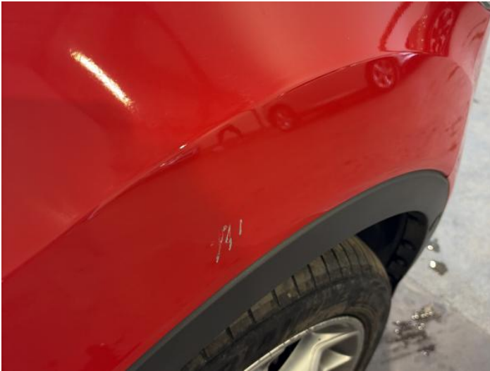
15: Wing osf Scratched Over 25mm Thru Paint
