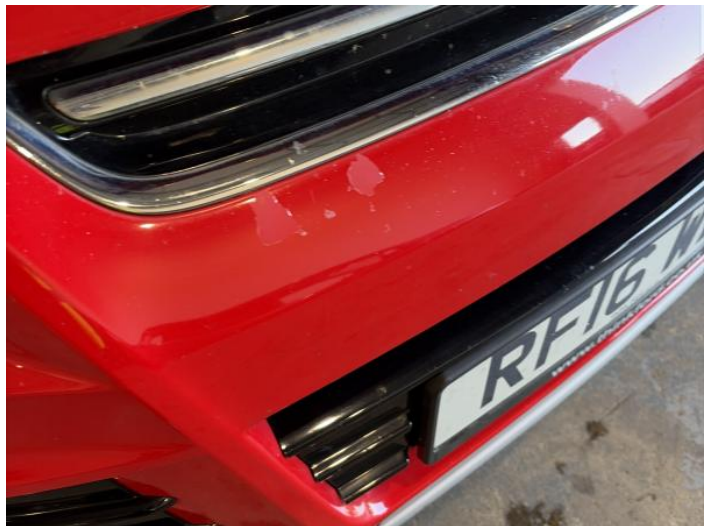
2: Bumper Front Poor Previous Repair Paint Flake
