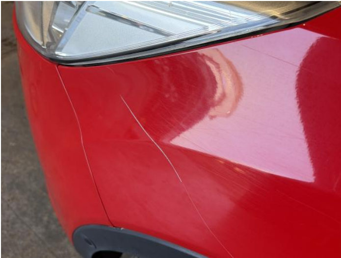
3: Wing nsf Scratched Over 25mm Thru Paint
