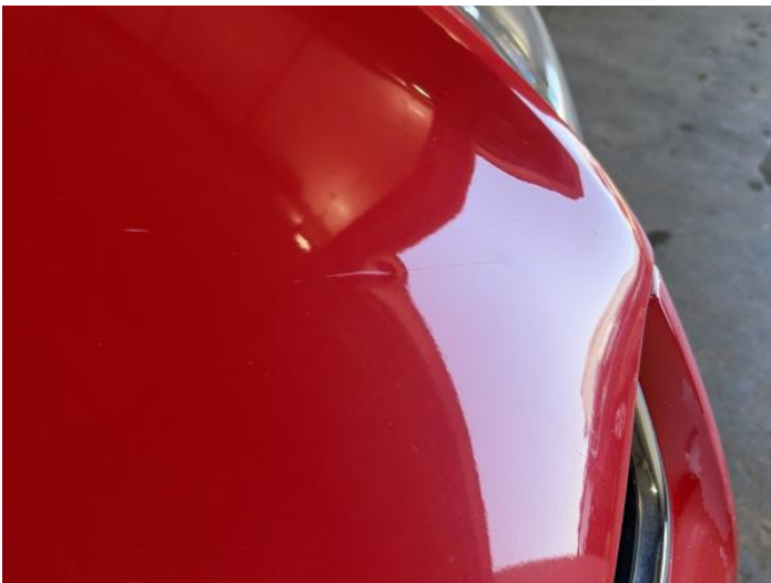
1: Bonnet Dented With Paint Damage
