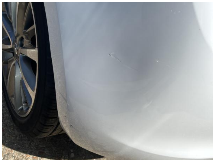
8: Bumper Rear Scratched 25 to 100mm Thru Paint
