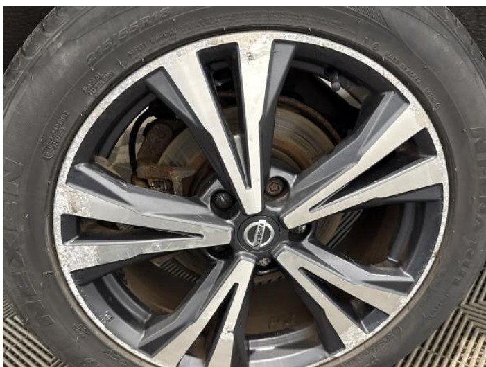
11: Wheel osr Scratched Over 50mm
