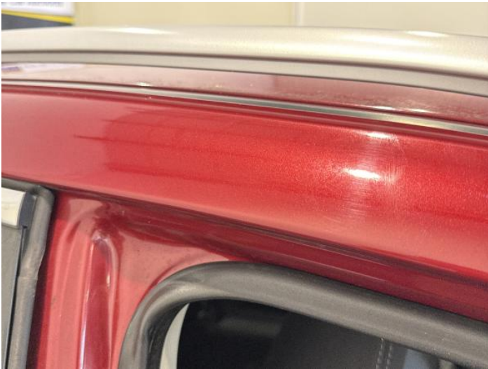
17: A Post os Poor Previous Repair Poor Paint
