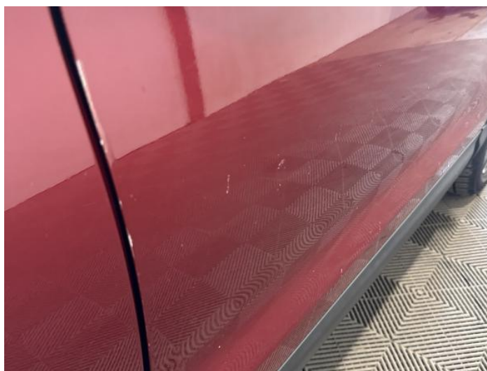
14: Door osf Scratched Over 25mm Thru Paint
