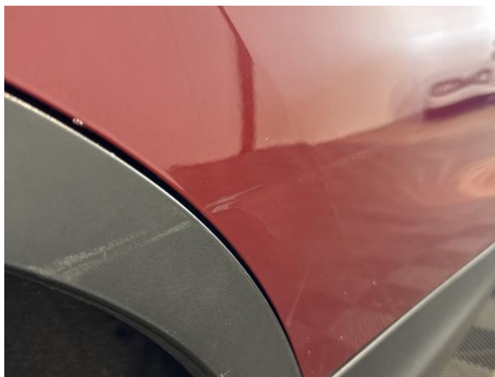
12: Door osr Dented With Paint Damage
