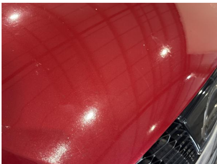
1: Bonnet Poor Previous Repair Poor Paint
