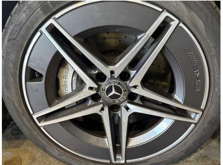
16: Wheel osf Scratched Over 50mm
