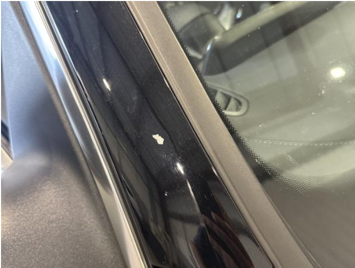
15: A Post os Dented With Paint Damage
