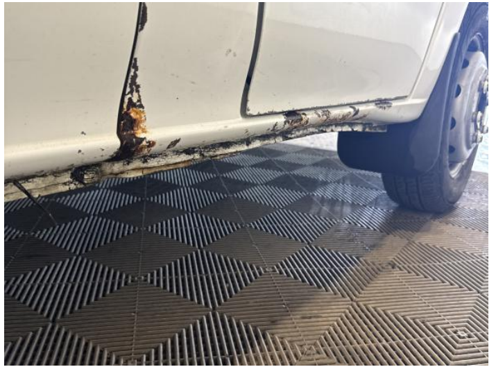
12: Sill os Rusted Over 5mm
