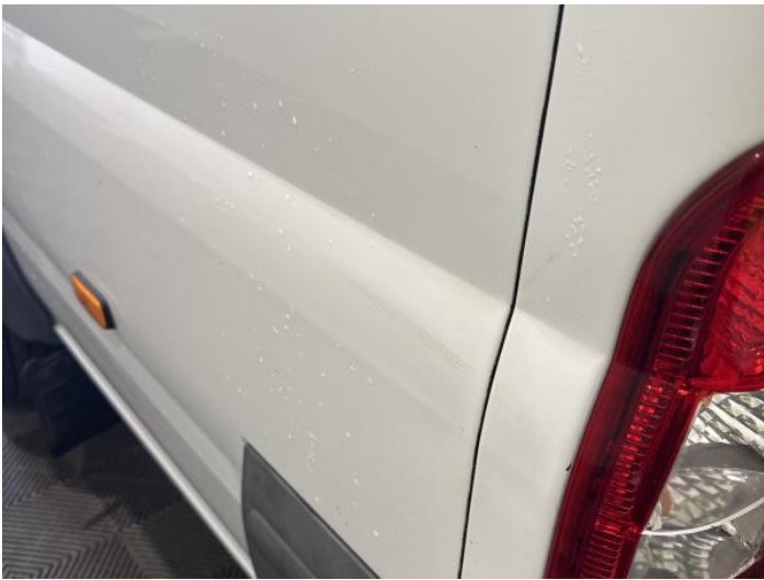
7: Qtr Panel nsr Dented With Paint Damage
