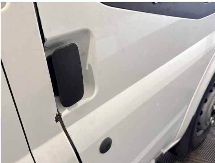
13: Door osf Dented With Paint Damage
