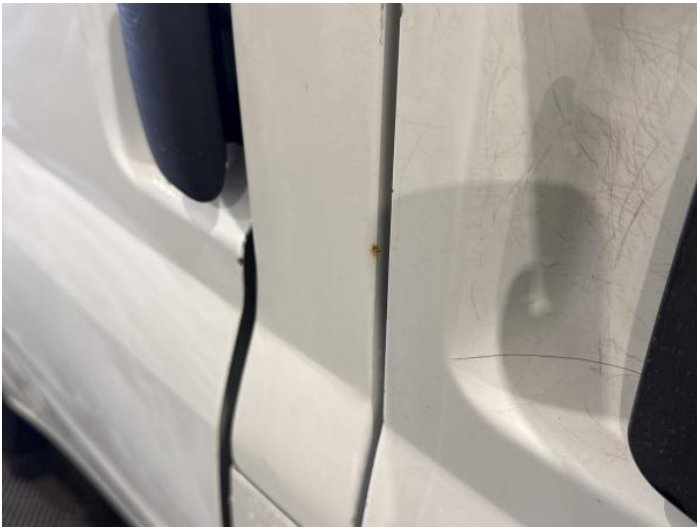
5: B Post ns Rusted Over 5mm
