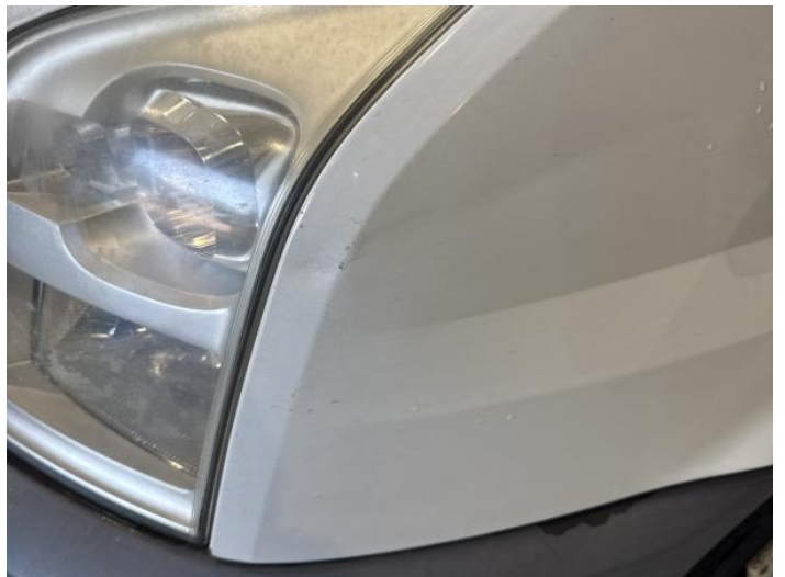
2: Wing nsf Dented With Paint Damage
