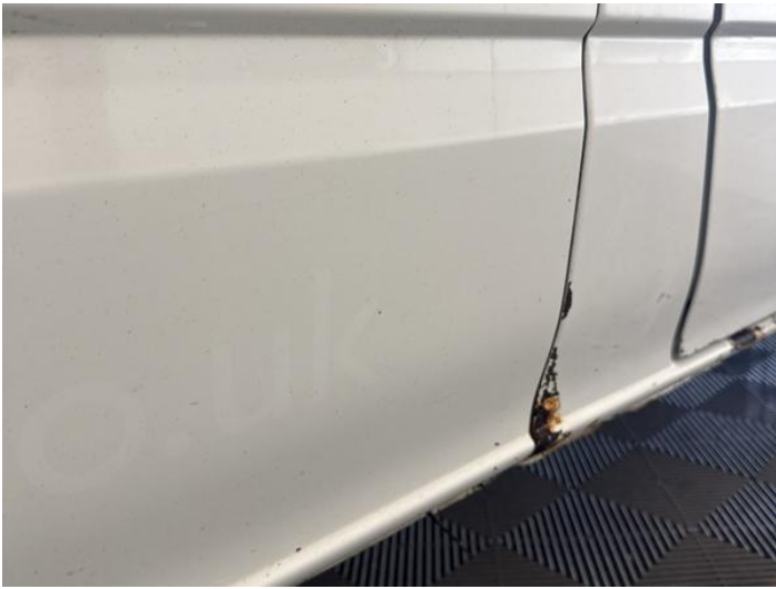
11: Panel Front Rusted Over 5mm
