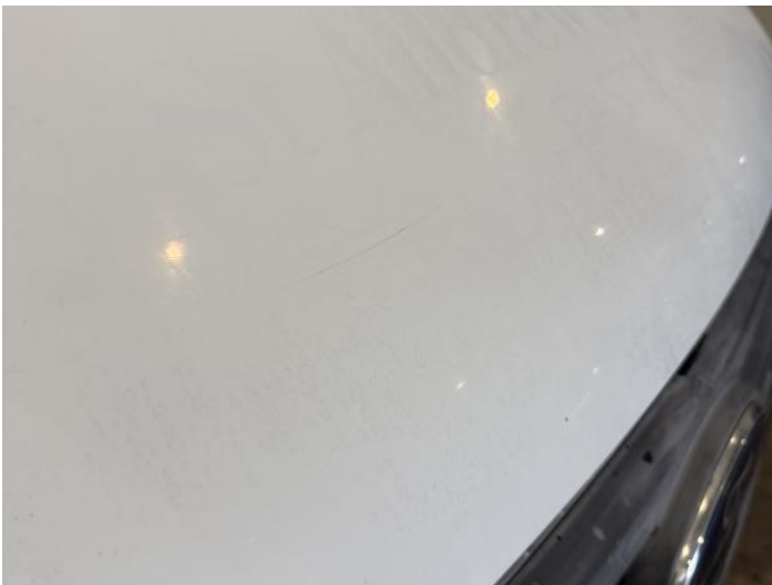
1: Bonnet Scratched Over 25mm Thru Paint
