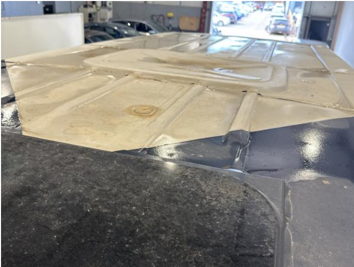
15: Roof Dented Over 30mm
