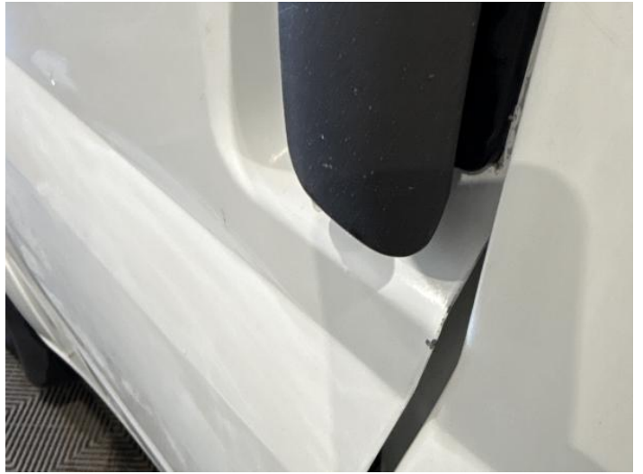
4: Door nsf Scratched UpTo 25mm Thru Paint
