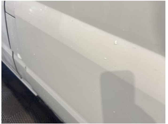
6: Door nsr Dented With Paint Damage
