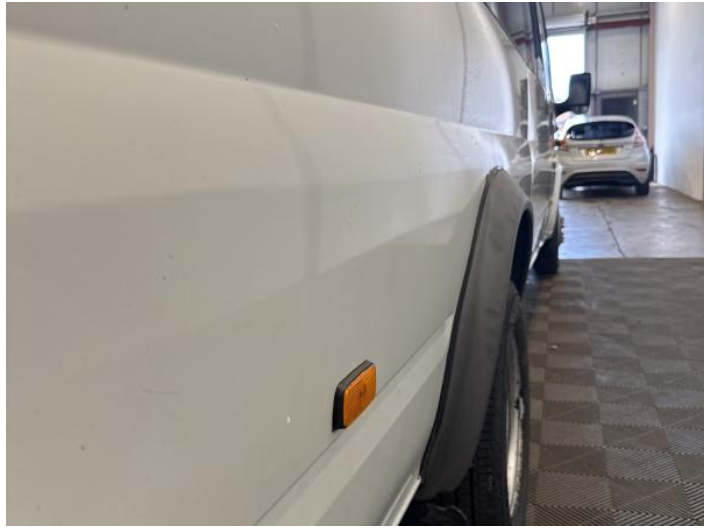
10: Qtr Panel osr Dented Over 30mm
