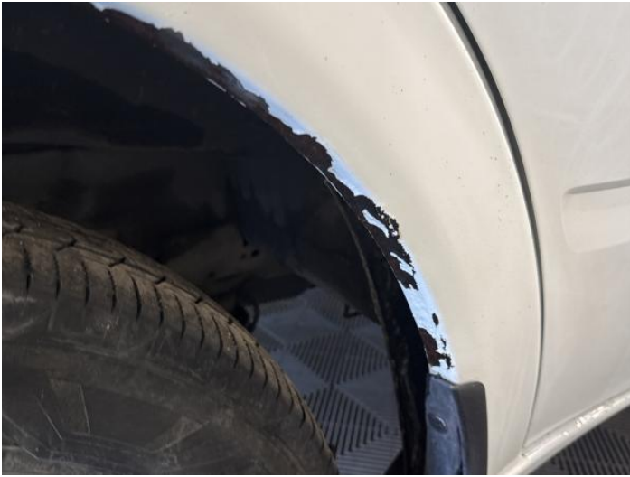
3: Wing nsf Rusted Over 5mm
