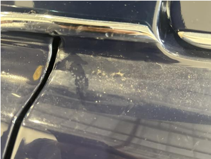
15: Wing osf Rusted Over 5mm
