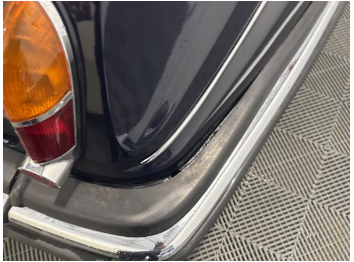
10: Bumper Rear Moulding Broken Replace
