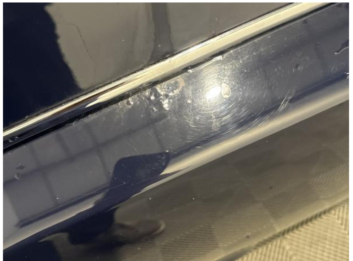
12: Qtr Panel osr Rusted UpTo 5mm
