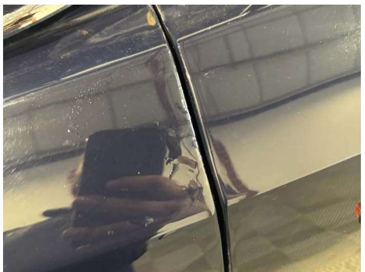
14: Door osf Rusted Over 5mm
