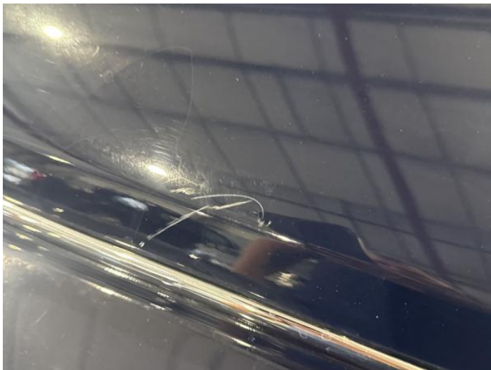
3: Boot Lid Scratched UpTo 25mm Thru Paint
