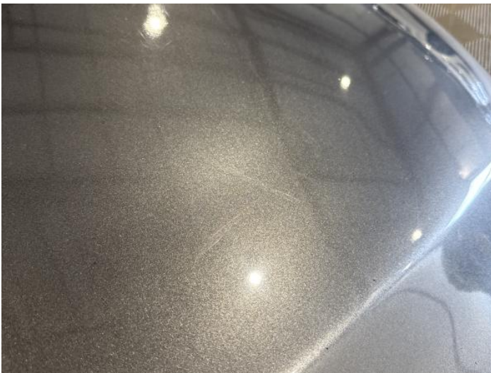
1: Bonnet Scratched Over 25mm Thru Paint
