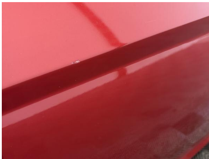
2: Door osf Chipped 1 To 5
