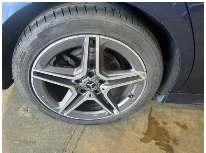
8: Wheel osr Corroded Light
