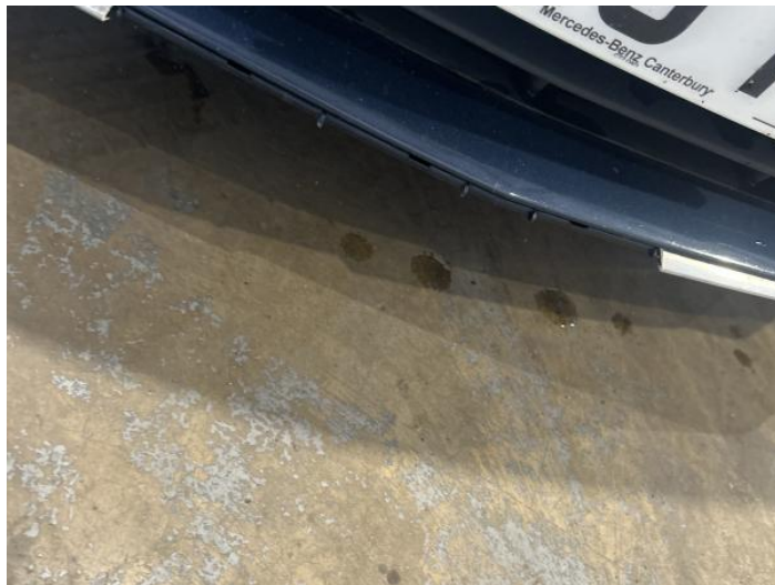
16: Bumper Front Moulding Broken Replace
