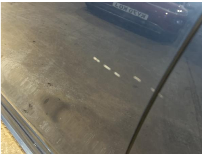
13: Door nsf Scratched Over 25mm Thru Paint
