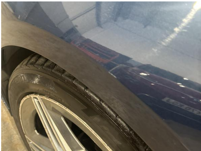
15: Wing nsf Scratched UpTo 25mm Thru Paint
