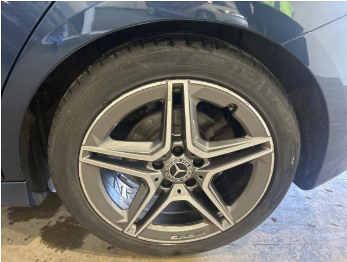
9: Wheel nsr Corroded Light
