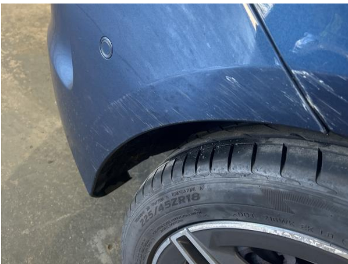
7: Bumper Rear Scratched Over 100mm Thru Paint
