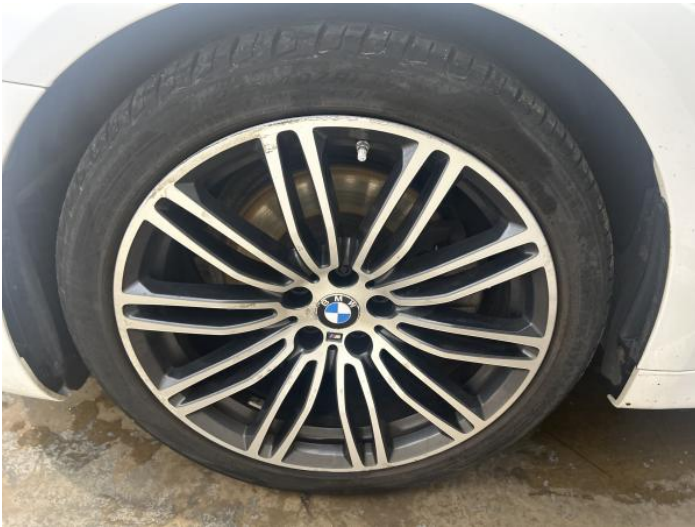
11: Wheel nsf Scratched Over 50mm
