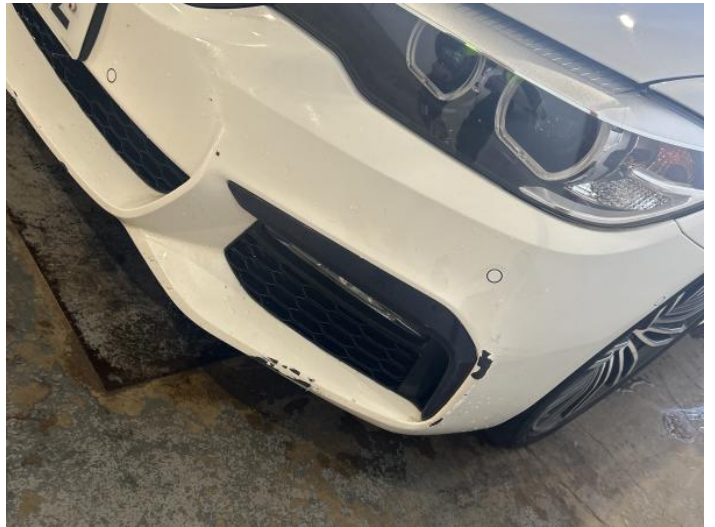
12: Bumper Front Scratched Over 100mm Thru Paint
