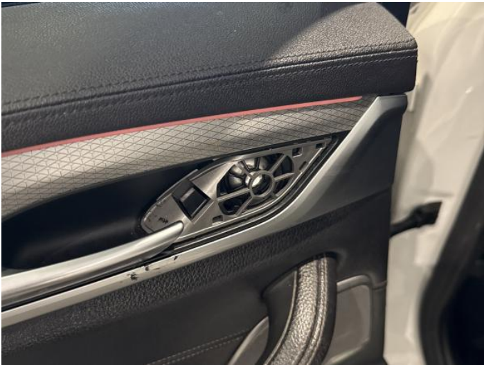
17: Fascia Trim Missing Replace
