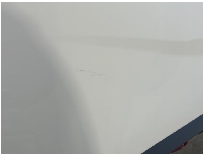
13: Bonnet Scratched UpTo 25mm Not Thru Paint
