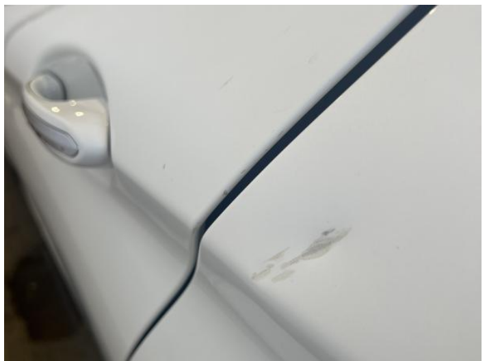
8: Door nsr Chipped Edge Chip
