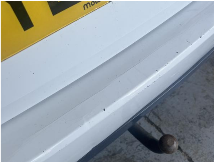
5: Bumper Rear Poor Previous Repair Paint Flake
