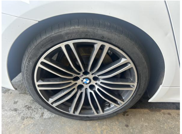
4: Wheel osr Scratched Over 50mm
