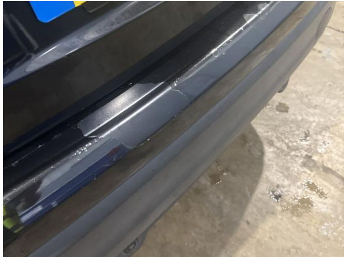
16: Bumper Rear Poor Previous Repair Paint Flake
