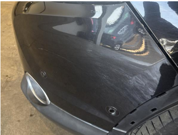
5: Bumper Front Scratched 25 to 100mm Thru Paint
