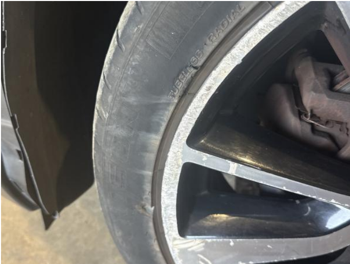
3: Tyre nsf Damaged Replace
