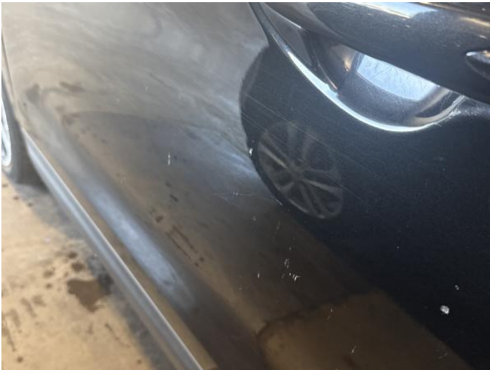
11: Door nsf Dented With Paint Damage
