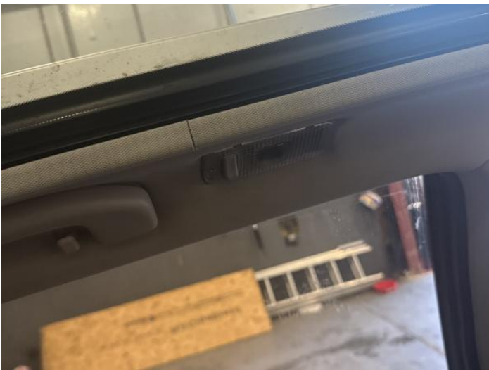
1: Roof Lining Scuffed Up To 25mm
