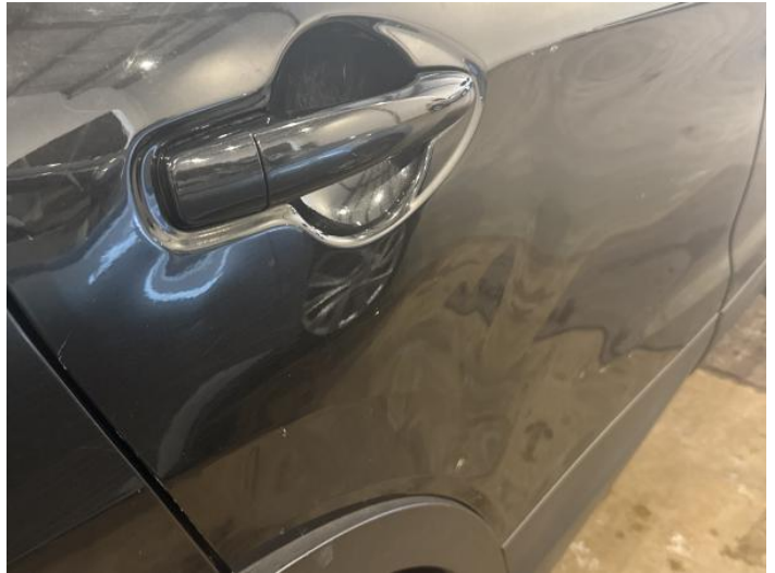
22: Door osr Dented With Paint Damage
