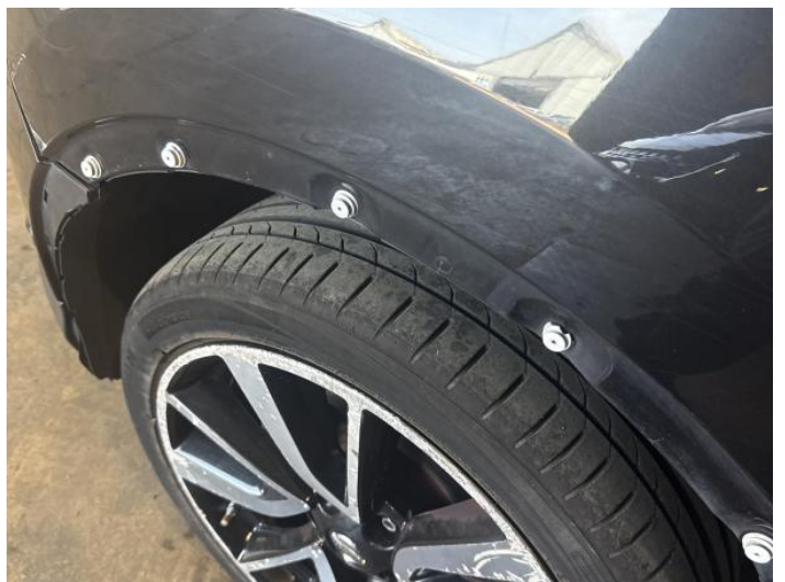
8: Wing Front Arch Extension ns Missing Replace
