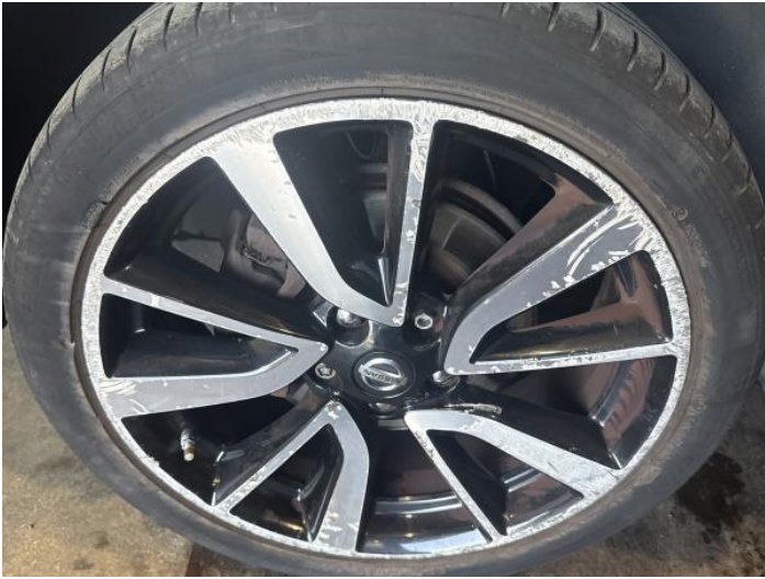
9: Wheel nsf Scratched Over 50mm
