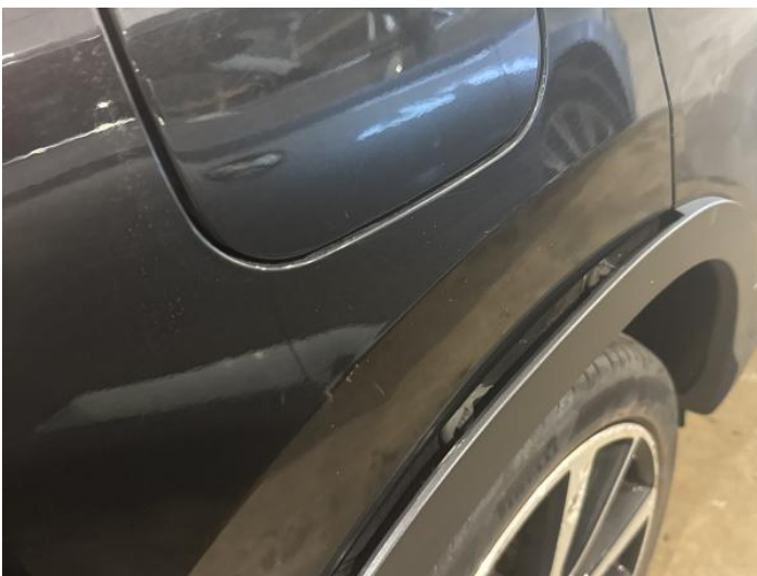
19: Qtr Panel osr Dented With Paint Damage
