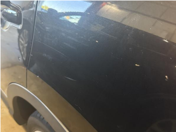
15: Qtr Panel nsr Scratched Over 25mm Thru Paint
