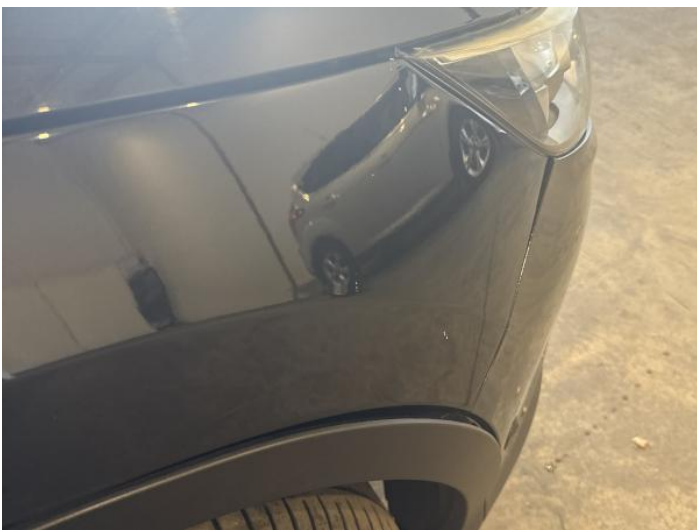
25: Wing osf Scratched Over 25mm Thru Paint
