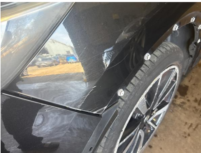
7: Wing nsf Dented With Paint Damage
