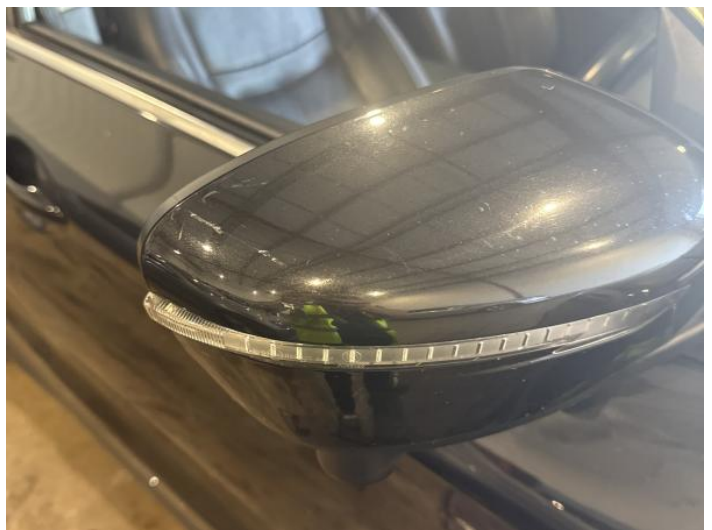
26: Door Mirror Assy osf Scratched (Painted) Over 25mm Thru Paint
