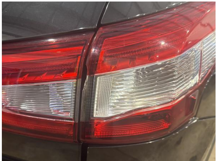
18: Lamp osr Broken Replace
