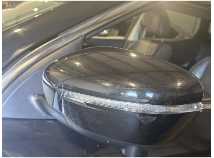
10: Door Mirror Assy nsf Broken Replace
