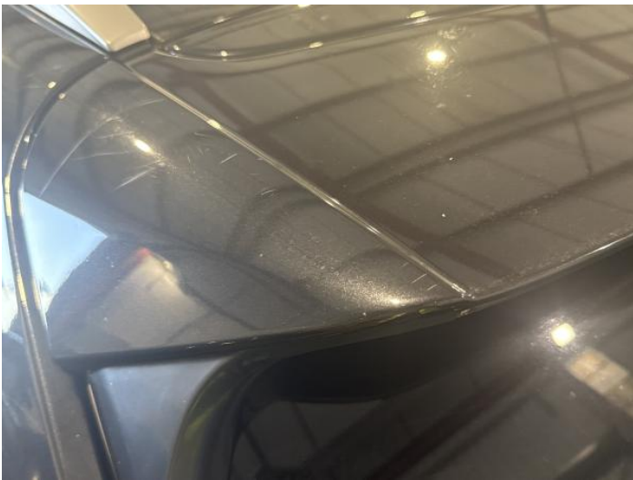
17: Spoiler Rear Scratched (Painted) Over 25mm Thru Paint
