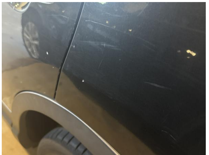
14: Qtr Panel nsr Dented Between 10mm + 30mm
