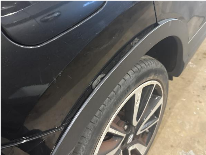
21: Qtr Panel Arch Extension os Broken Replace
