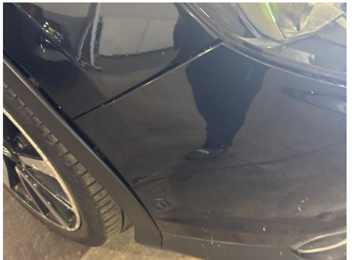
6: Bumper Front Insecure Action Required
