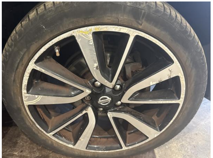
24: Wheel osf Scratched Over 50mm
