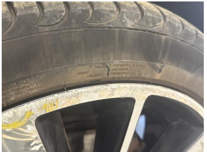
2: Tyre osf Damaged Replace
