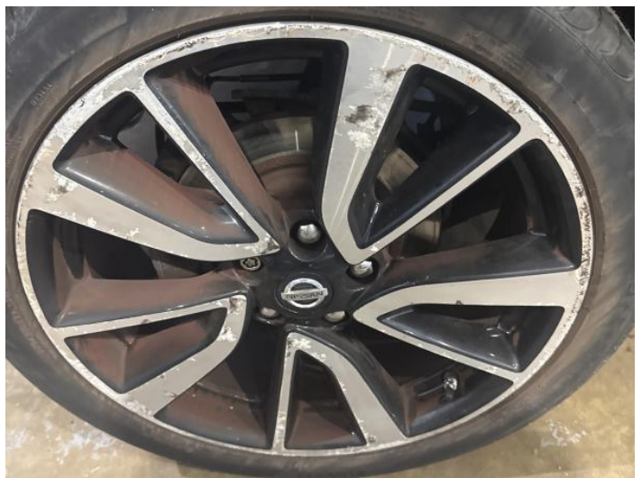
20: Wheel osr Scratched Over 50mm
