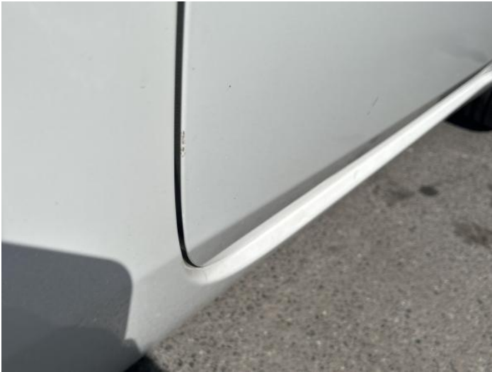
3: Door osf Chipped Edge Chip
