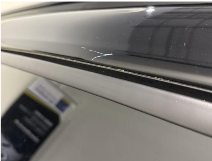
17: B Post os Scratched Over 25mm Thru Paint
