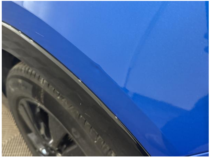
6: Qtr Panel nsr Dented Between 10mm + 30mm
