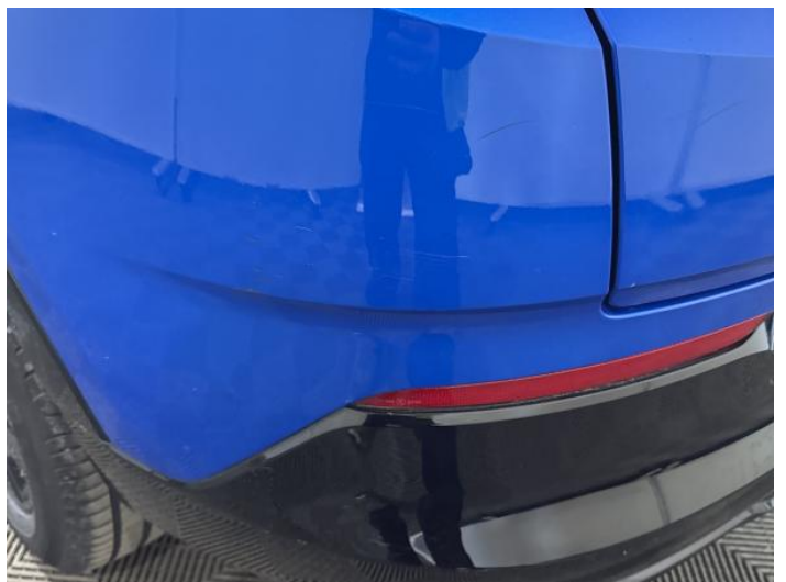
8: Bumper Rear Scratched 25 to 100mm Thru Paint
