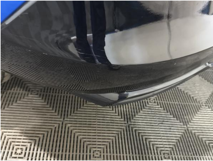
9: Bumper Rear Moulding Scratched (Painted) Over 25mm Thru Paint
