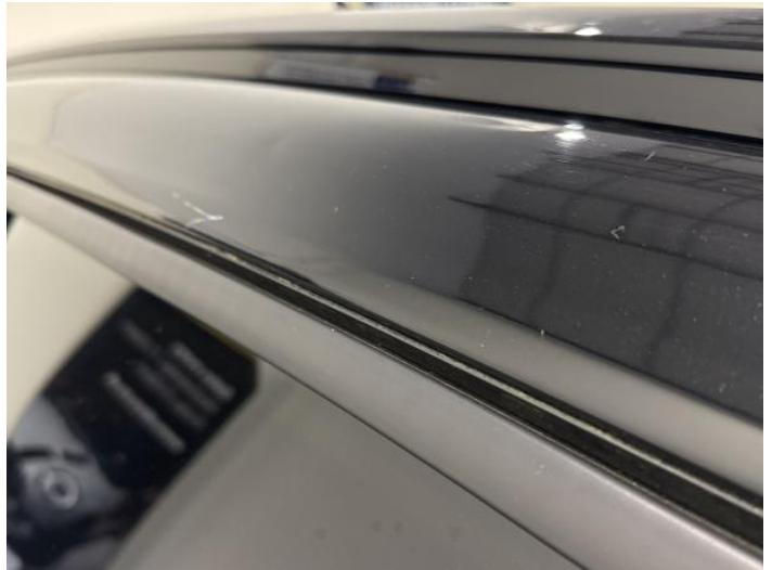
16: B Post os Dented Between 10mm + 30mm
