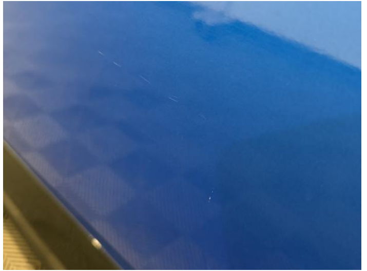
4: Door nsf Scratched UpTo 25mm Thru Paint
