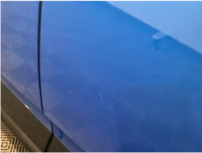
5: Door nsr Scratched UpTo 25mm Thru Paint
