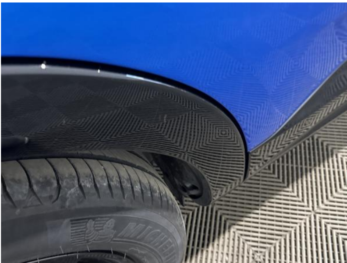
11: Qtr Panel Arch Extension os Scratched (Painted) UpTo 25mm Thru Paint
