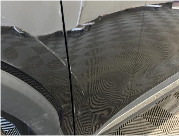
9: Door nsf Scratched Over 25mm Thru Paint
