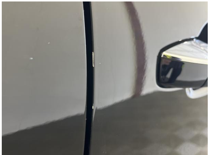
2: Door osf Chipped Edge Chip
