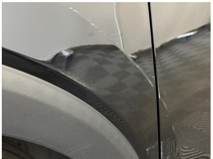
8: Wing nsf Scratched Over 25mm Thru Paint
