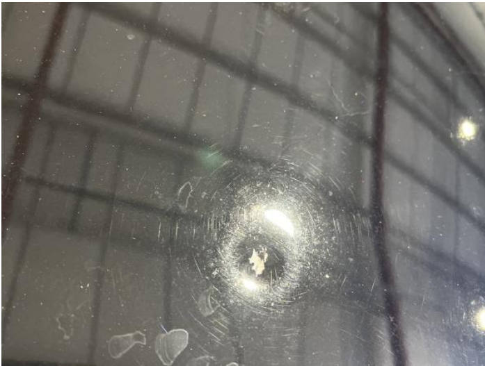
5: Bonnet Dented With Paint Damage
