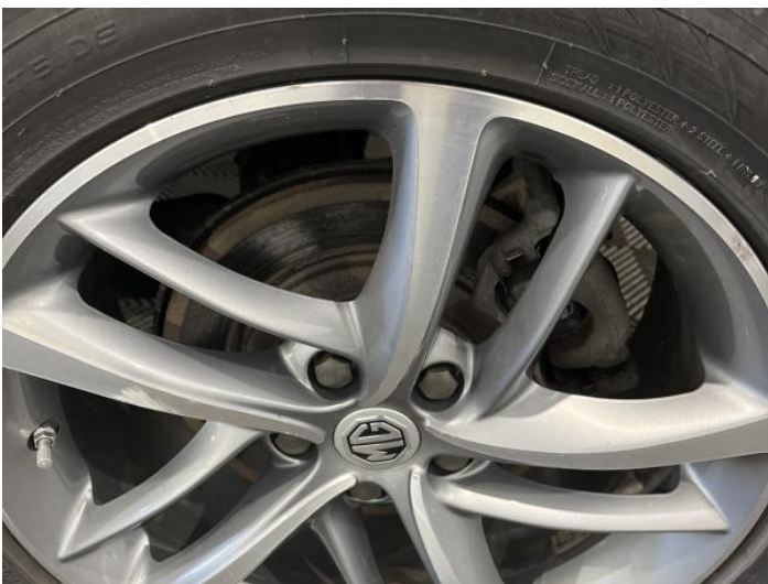
13: Wheel nsr Corroded Light
