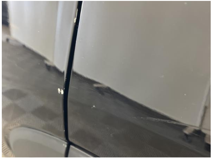
12: Qtr Panel nsr Dented Over 2 UpTo 10mm
