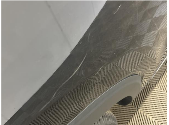
16: Door osr Dented With Paint Damage
