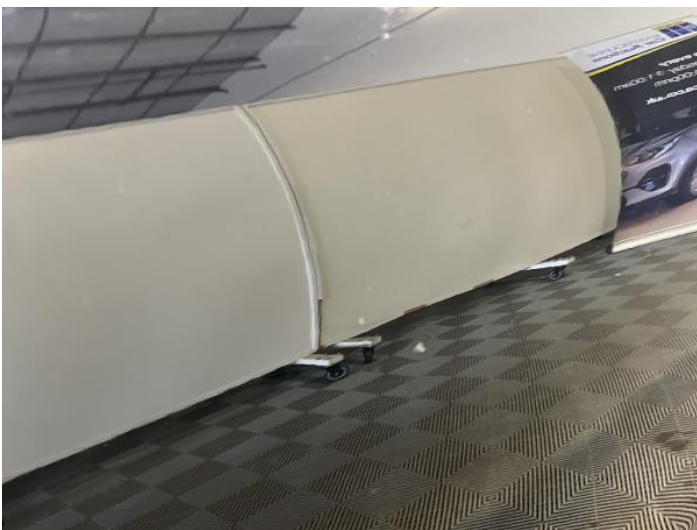
7: Door nsf Dented With Paint Damage
