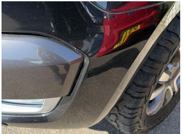
2: Bumper Front Scratched 25 to 100mm Thru Paint
