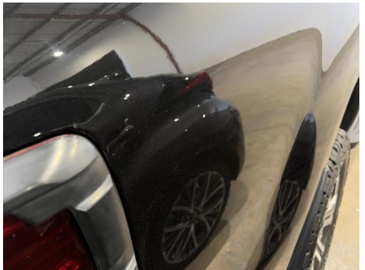
12: Qtr Panel osr Poor Previous Repair Poor Paint
