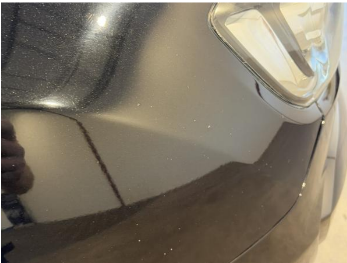
17: Wing osf Chipped Multiple Chips
