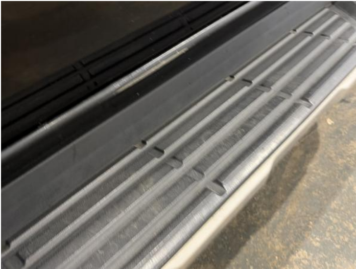
15: Sill os Scratched Over 25mm Thru Paint
