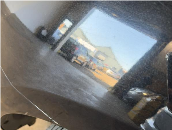
3: Wing nsf Scratched Over 25mm Thru Paint
