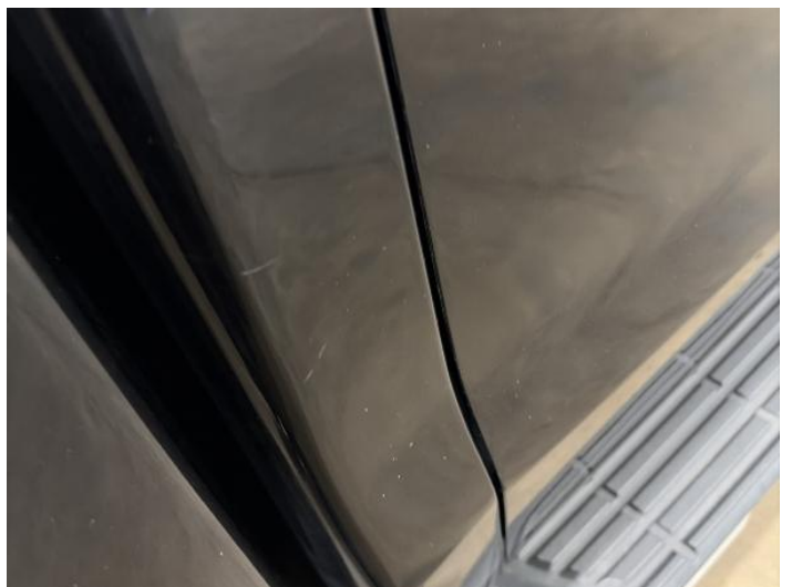
14: C Post os Scratched Up To 25mm Thru Paint
