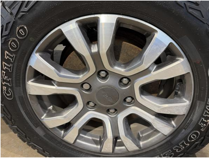
9: Wheel nsr Scratched Up To 50mm
