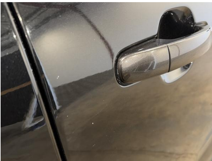
13: Door osr Scratched Over 25mm Thru Paint
