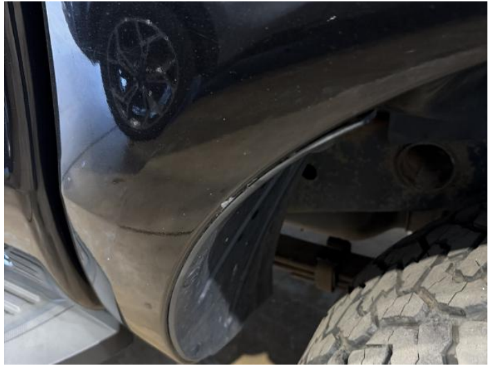
10: Qtr Panel nsr Chipped Over 5mm
