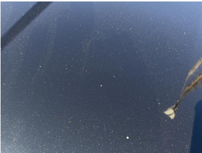
1: Bonnet Scratched Over 25mm Thru Paint
