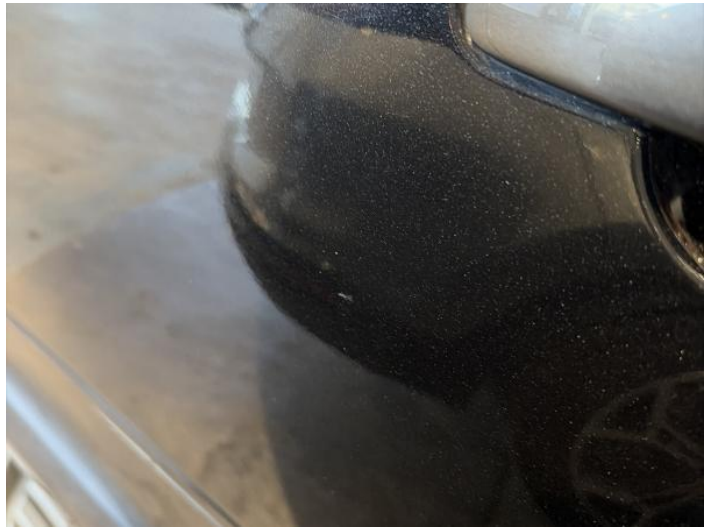
6: Door nsf Dented Between 10mm + 30mm
