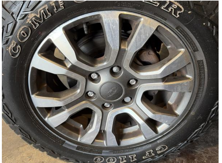
4: Wheel nsf Scratched Over 50mm
