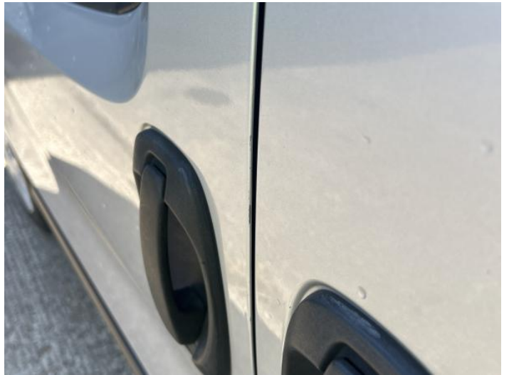
6: Door nsf Chipped Edge Chip
