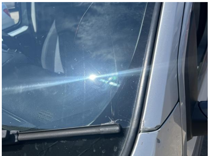
8: Screen Front Cracked Replace
