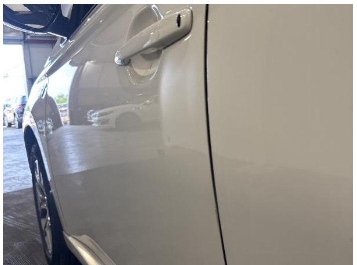
8: Door nsf Dented Over 30mm
