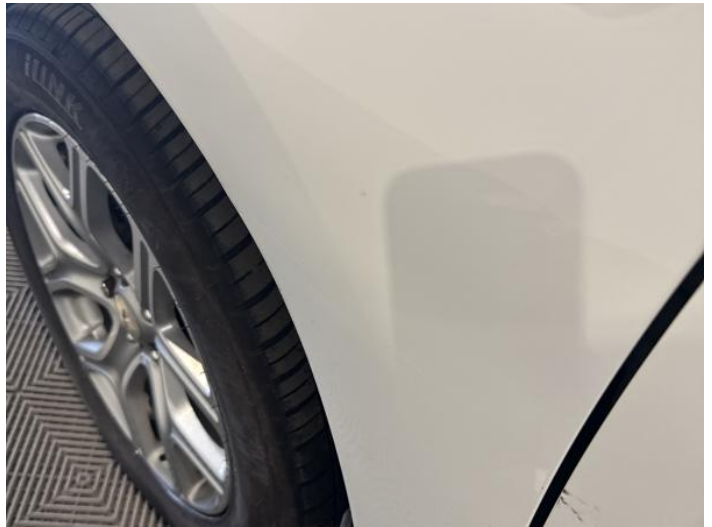
6: Wing nsf Scratched Over 25mm Thru Paint
