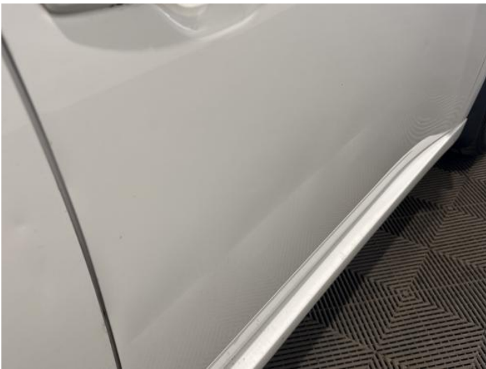
17: Door osf Dented Over 30mm
