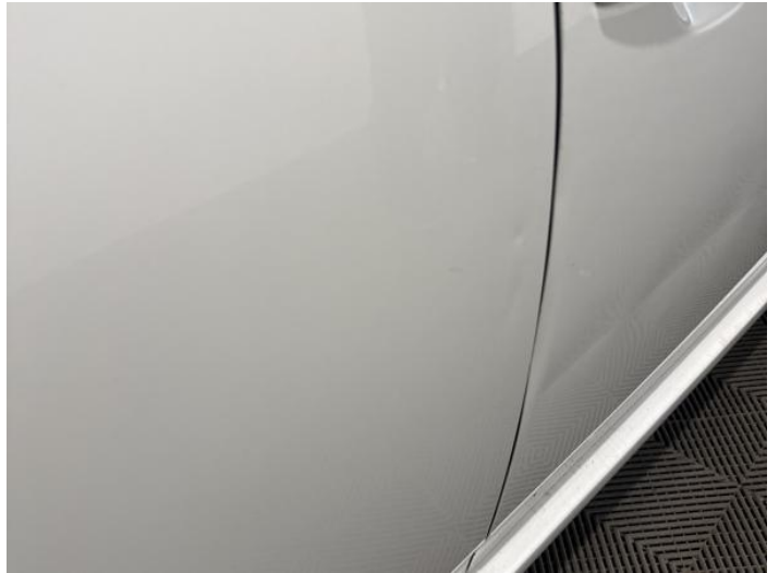
16: Door osr Dented Over 30mm
