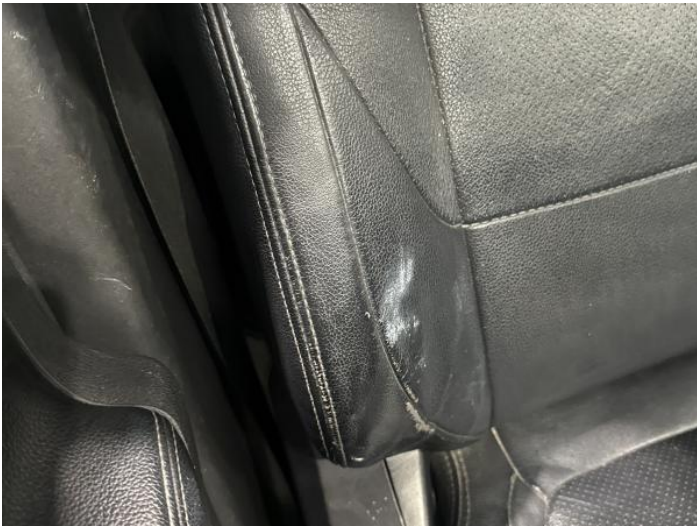
1: Seat Back Cover osf Scuffed Over 25mm
