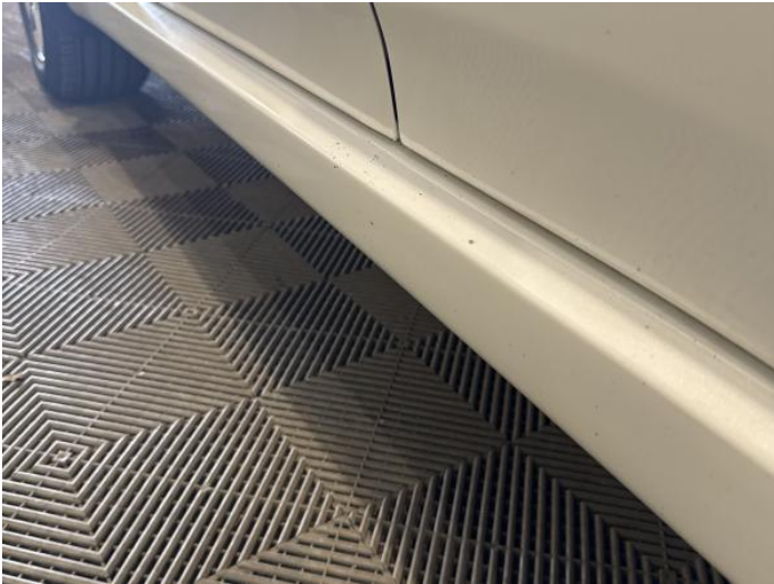
9: Sill Panel Trim ns Scratched (Painted) Over 25mm Thru Paint
