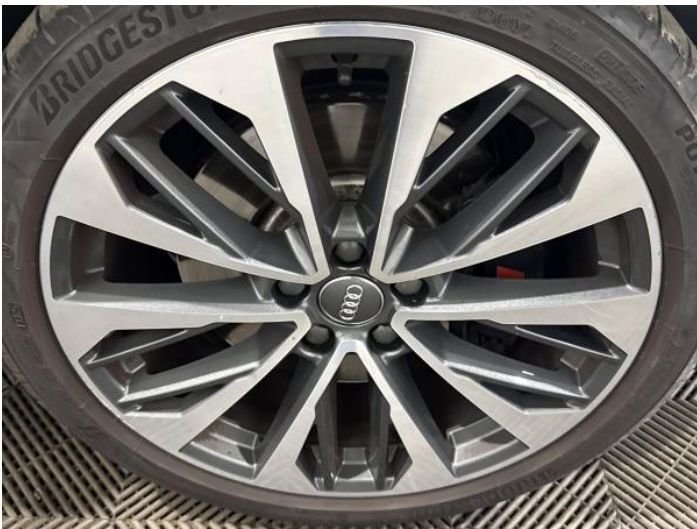
11: Wheel osf Scratched Over 50mm
