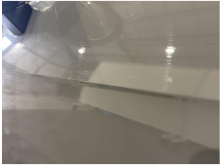
4: Door nsf Dented Between 10mm + 30mm
