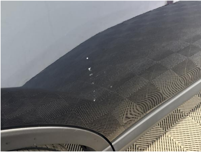
9: Door osr Scratched Over 25mm Thru Paint
