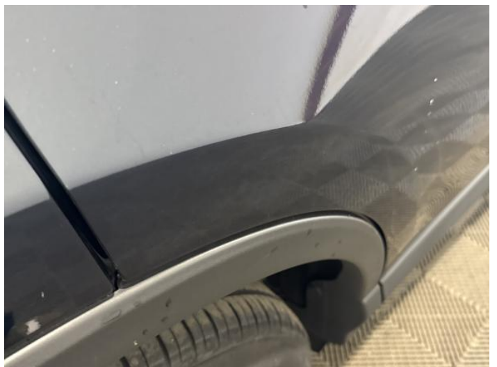
8: Door osr Dented Between 10mm + 30mm
