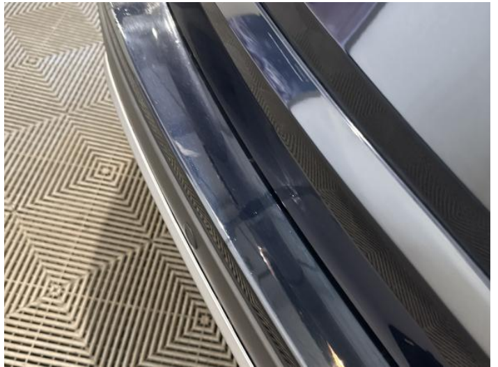
6: Bumper Rear Scratched 25 to 100mm Thru Paint
