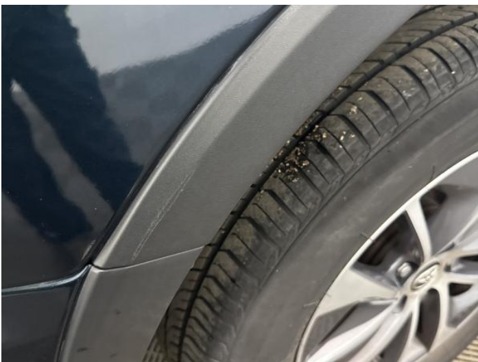
7: Qtr Panel Arch Extension os Scuffed (Unpainted) Over 100mm
