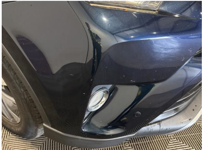
2: Bumper Front Scratched 25 to 100mm Thru Paint
