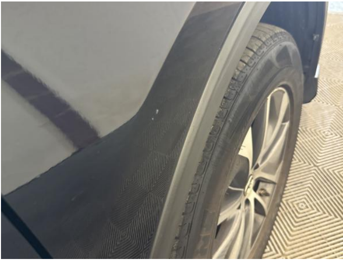
11: Wing osf Dented Between 10mm + 30mm
