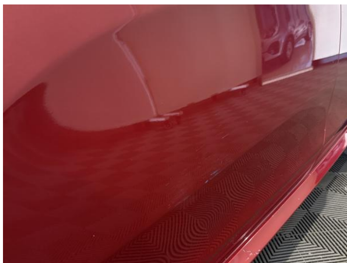
8: Door nsf Dented With Paint Damage
