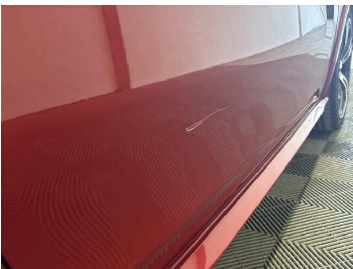
19: Door osf Dented With Paint Damage
