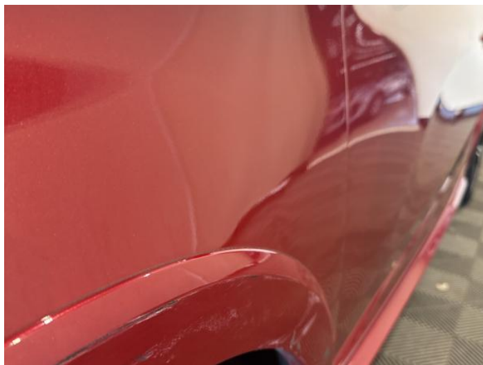
4: Wing nsf Dented Over 30mm
