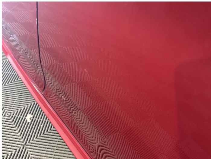
10: Qtr Panel nsr Dented Between 10mm + 30mm
