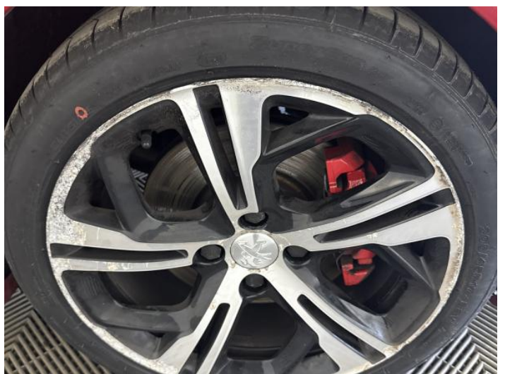
20: Wheel osf Scratched Over 50mm
