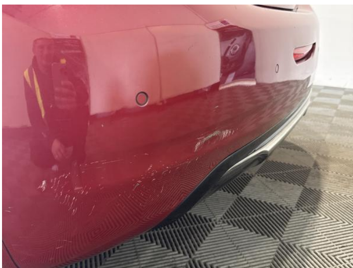
13: Bumper Rear Scratched Over 100mm Thru Paint
