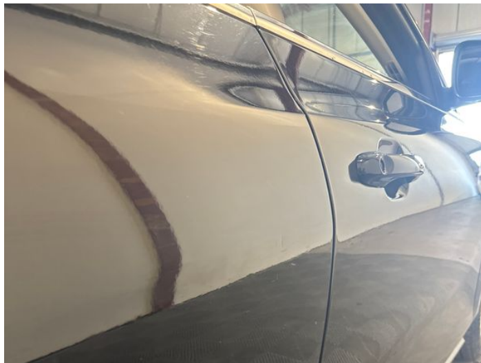
16: Door osr Dented With Paint Damage
