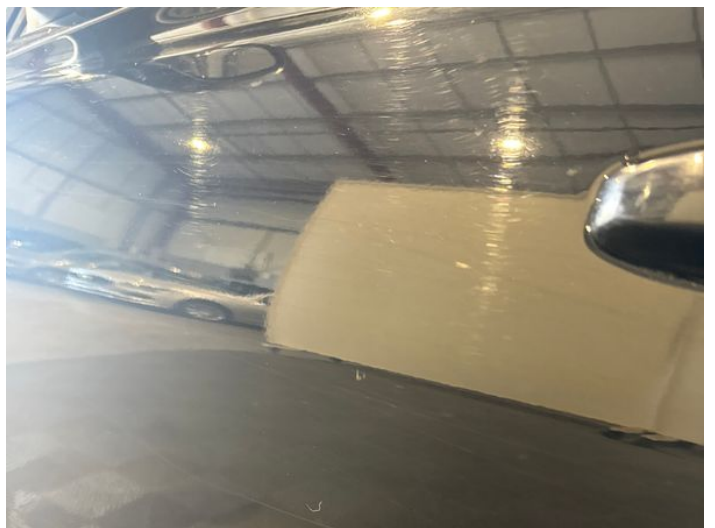
8: Door nsf Scratched Over 25mm Thru Paint
