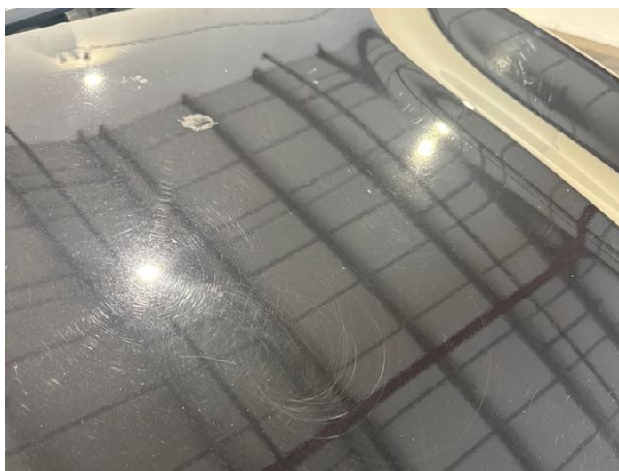
2: Bonnet Scratched Over 25mm Thru Paint
