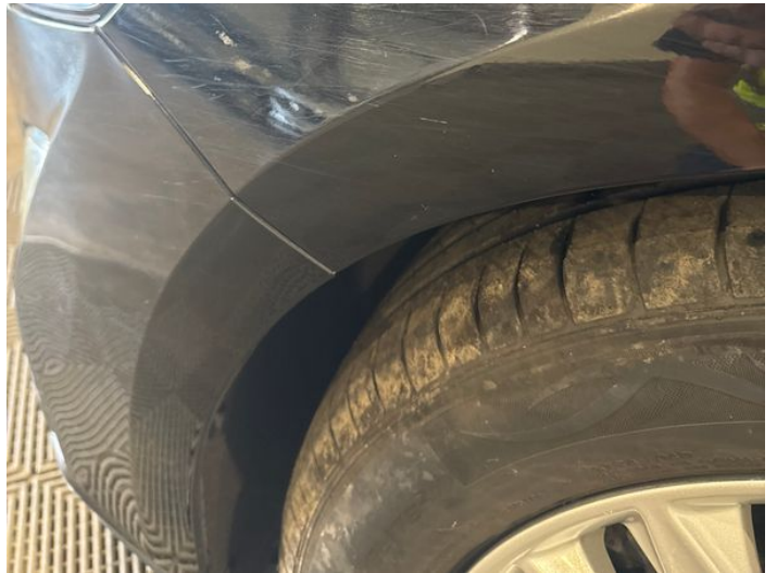
6: Wing nsf Scratched Over 25mm Thru Paint
