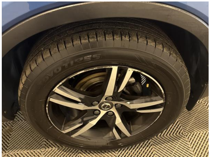
18: Wheel osf Scratched Over 50mm
