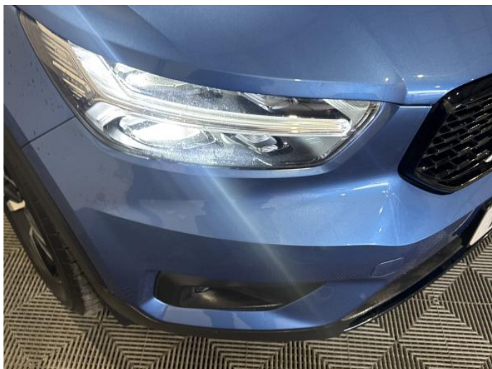
3: Bumper Front Scratched 25 to 100mm Thru Paint
