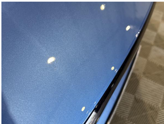
2: Bonnet Dented Over 2 UpTo 10mm
