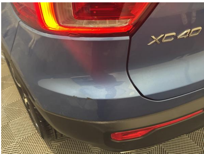
11: Bumper Rear Scratched 25 to 100mm Thru Paint
