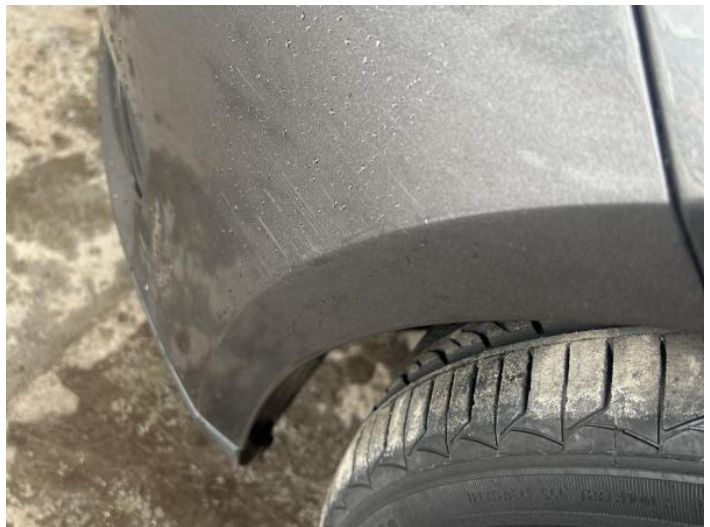
10: Bumper Front Scratched Over 25mm Not Thru Paint
