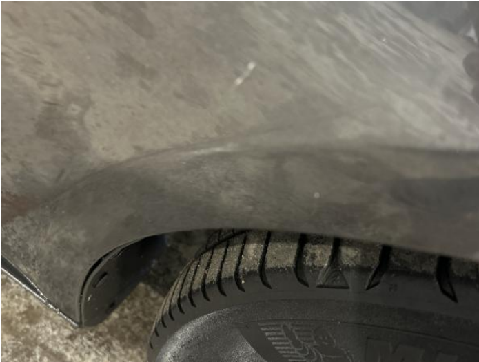
3: Wing osf Chipped 1 To 5
