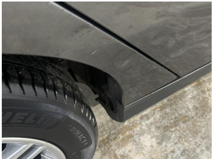
6: Qtr Panel osr Dented Over 30mm
