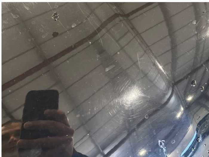
1: Bonnet Scratched Over 25mm Thru Paint
