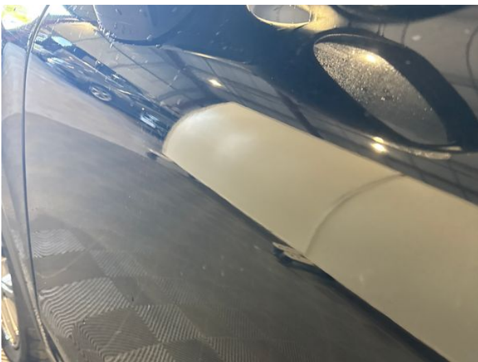
7: Door nsf Dented Over 30mm
