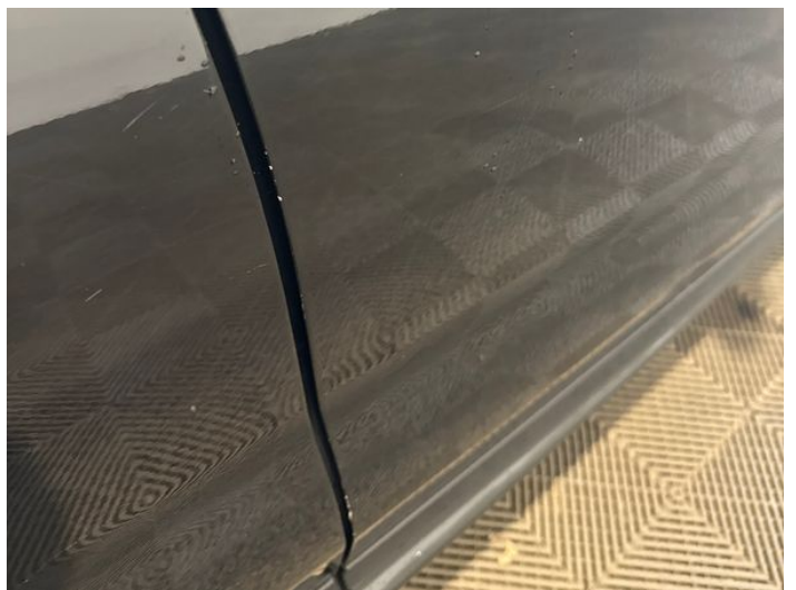
14: Door osf Chipped Edge Chip
