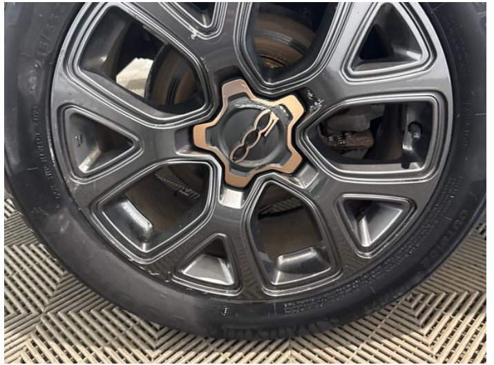
12: Wheel osr Scratched Over 50mm
