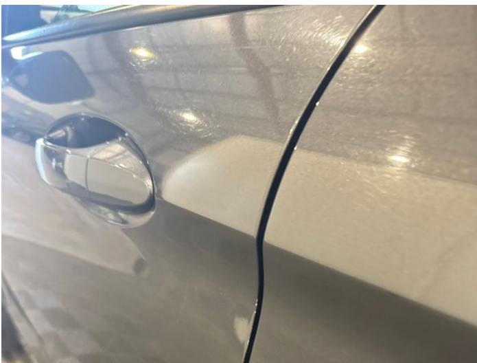
7: Door nsf Dented Over 30mm
