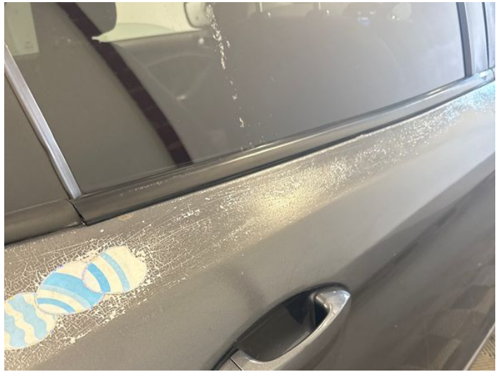
12: Door osr Poor Previous Repair Poor Paint
