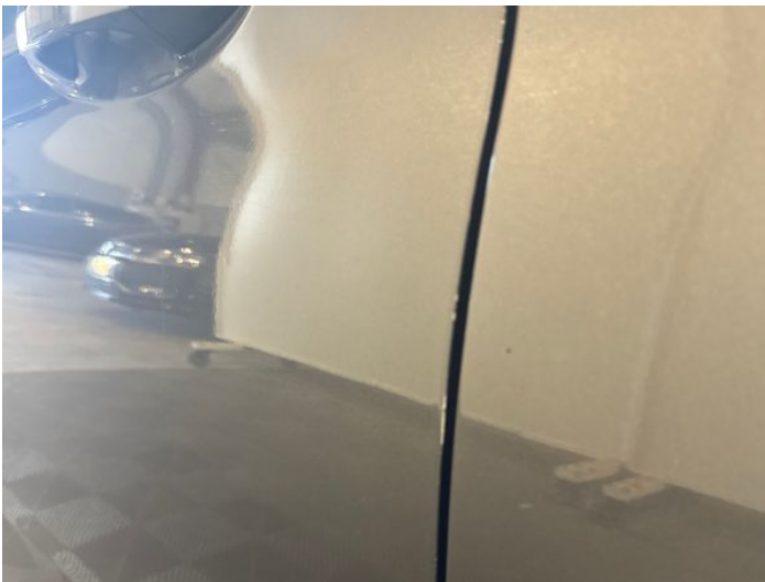
5: Door nsf Chipped Edge Chip
