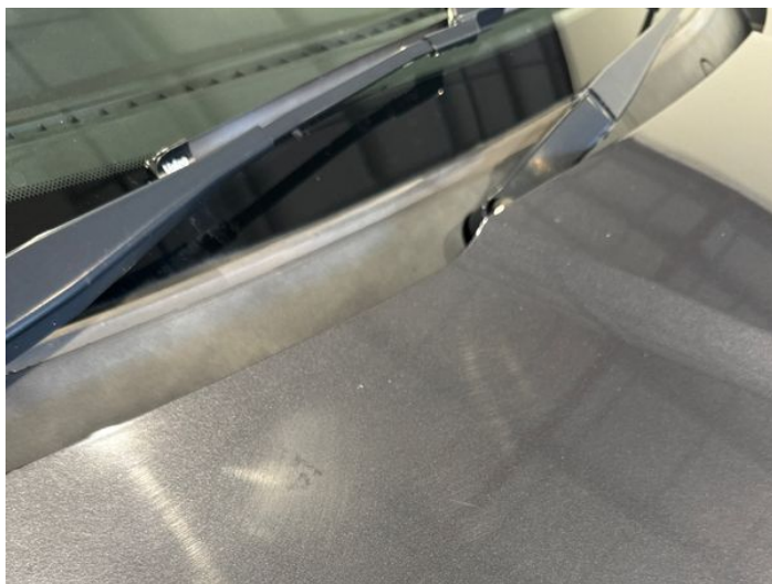
1: Bonnet Scratched Over 25mm Thru Paint
