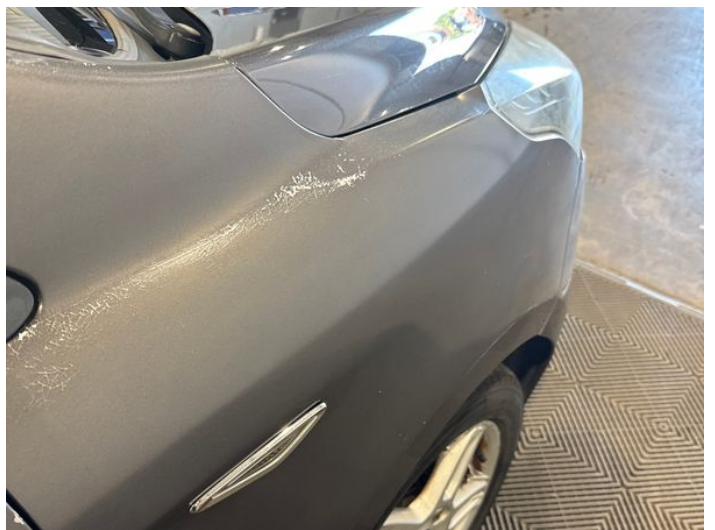
14: Wing osf Poor Previous Repair Poor Paint
