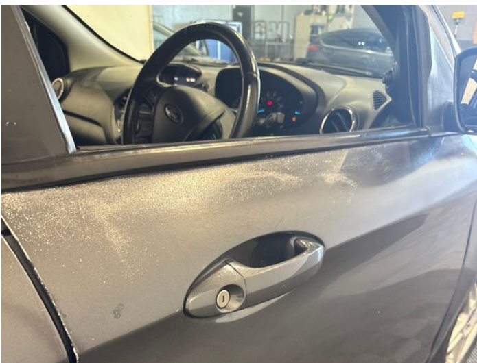
13: Door osf Poor Previous Repair Rippled UpTo 30%
