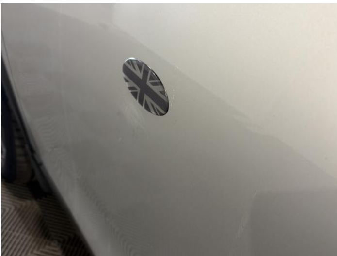
7: Door nsf Scratched Over 25mm Thru Paint
