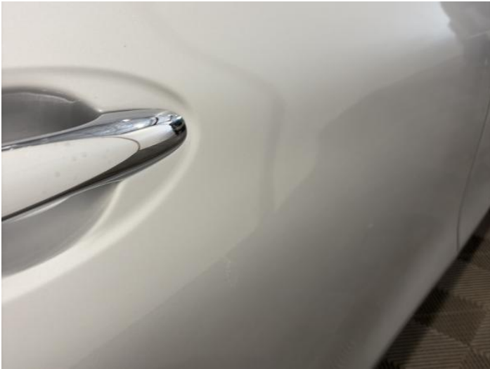
15: Door osr Poor Previous Repair Rippled UpTo 30%
