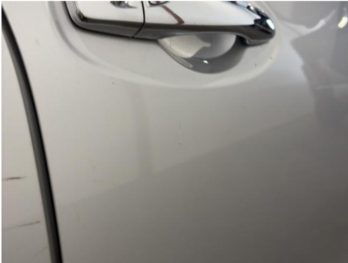
16: Door osf Scratched UpTo 25mm Thru Paint
