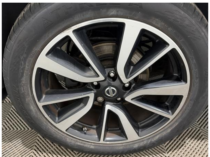
14: Wheel osr Scratched Over 50mm
