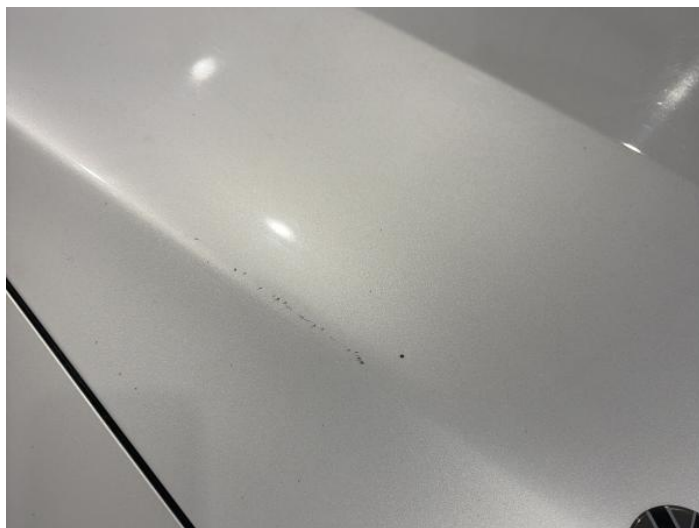
2: Bonnet Poor Previous Repair Poor Paint
