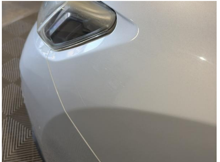
6: Wing nsf Scratched Over 25mm Thru Paint
