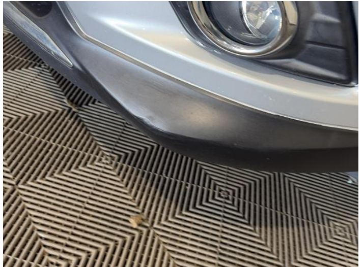
4: Bumper Front Moulding Scuffed (Unpainted) Over 100mm
