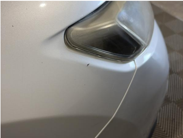
17: Wing osf Scratched UpTo 25mm Thru Paint
