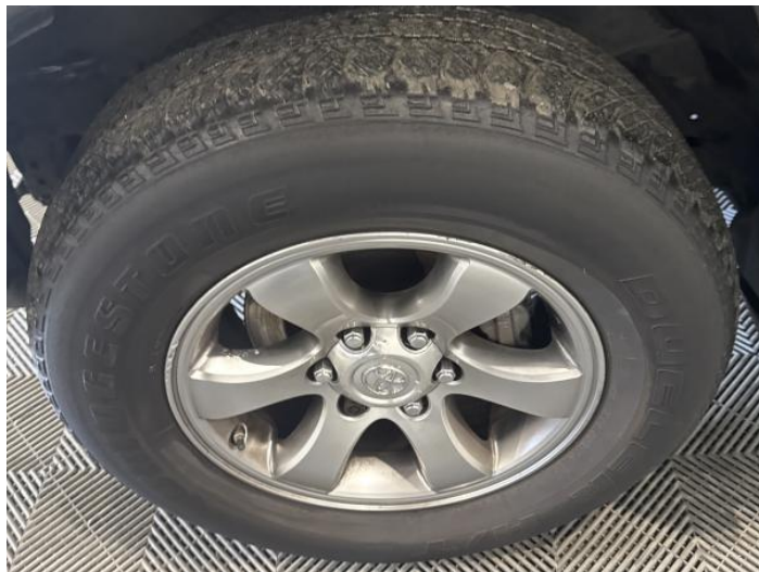
4: Wheel nsf Scratched Over 50mm
