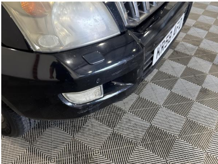
3: Bumper Front Scratched Over 100mm Thru Paint
