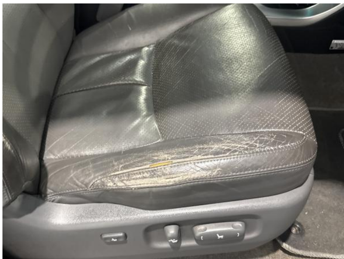
1: Seat Base Cover osf Torn Over 3mm
