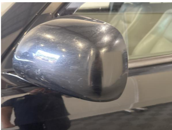
7: Door Mirror Assy nsf Scratched (Painted) Over 25mm Not Thru Paint
