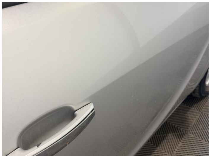
20: Door osf Dented With Paint Damage
