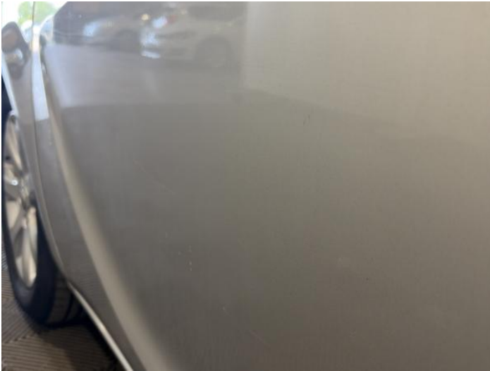
9: Door nsf Dented With Paint Damage
