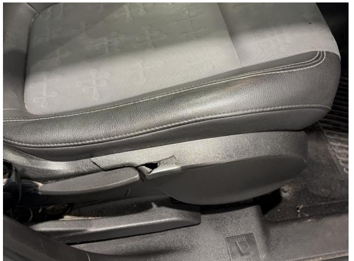
24: Fascia Trim Damaged Replace
