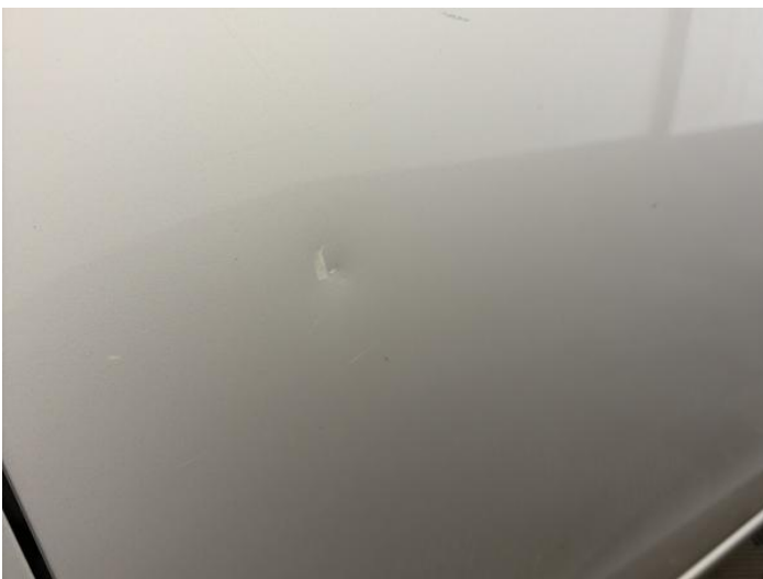
19: Door osr Dented With Paint Damage
