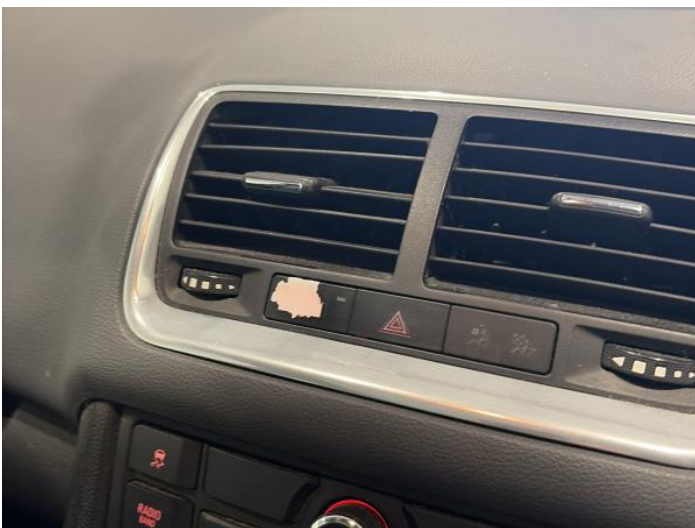
25: Switches And Controls Broken Replace
