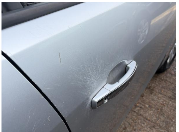
26: Door osf Scratched Over 25mm Thru Paint
