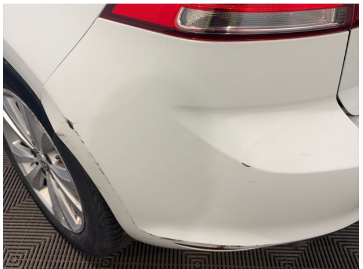
14: Bumper Rear Dented With Paint Damage
