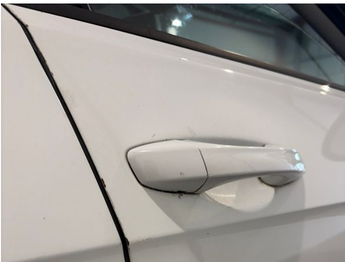
19: Door osf Scratched Rusted
