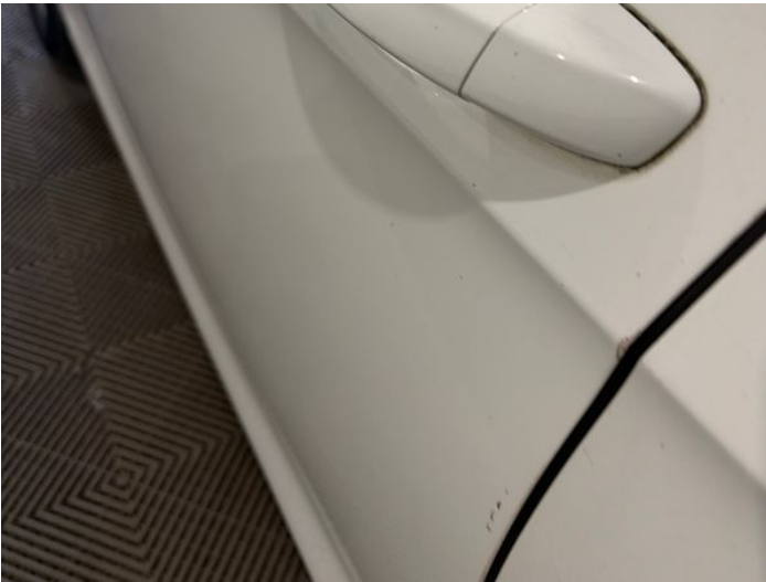
11: Door nsf Poor Previous Repair Rippled UpTo 30%
