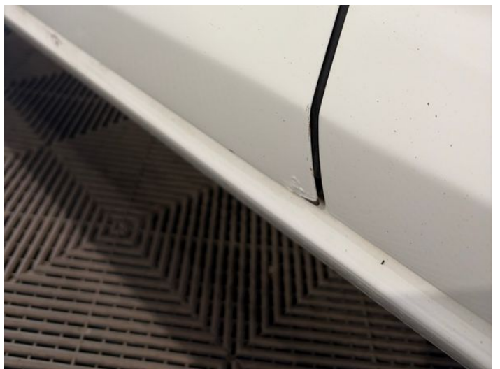
8: Door nsf Rusted Over 5mm
