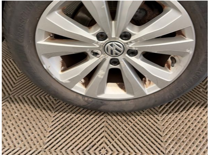
16: Wheel osr Scratched Over 50mm
