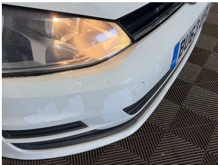
2: Bumper Front Poor Previous Repair Paint Flake
