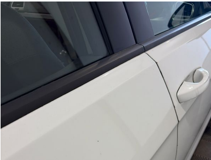
17: Door osr Dented Between 10mm + 30mm
