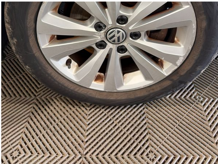
21: Wheel of Scratched Over 50mm
