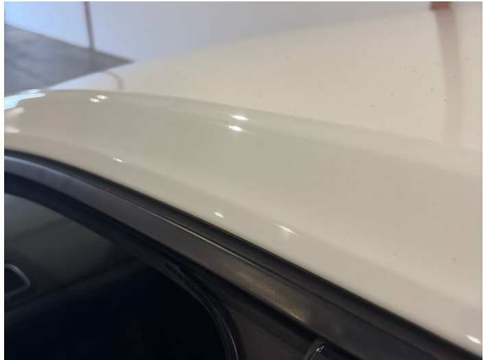
10: A Post ns Poor Previous Repair Poor Paint
