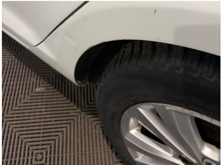
12: Qtr Panel nsr Dented With Paint Damage
