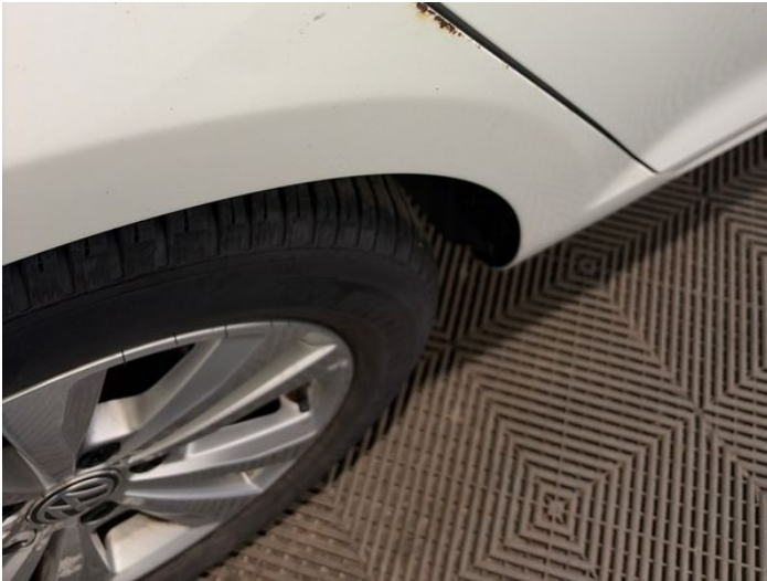
15: Qtr Panel osr Dented With Paint Damage
