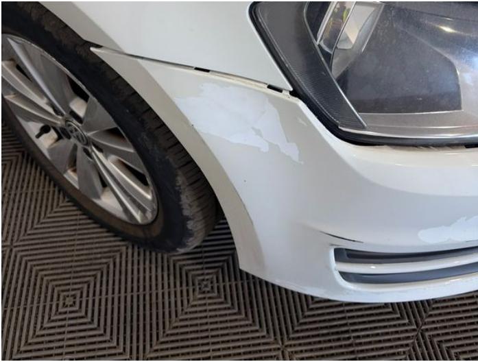
3: Bumper Front Insecure Action Required
