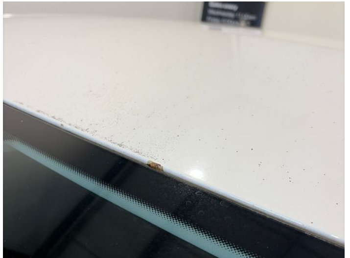
6: Roof Chipped Over 5mm
