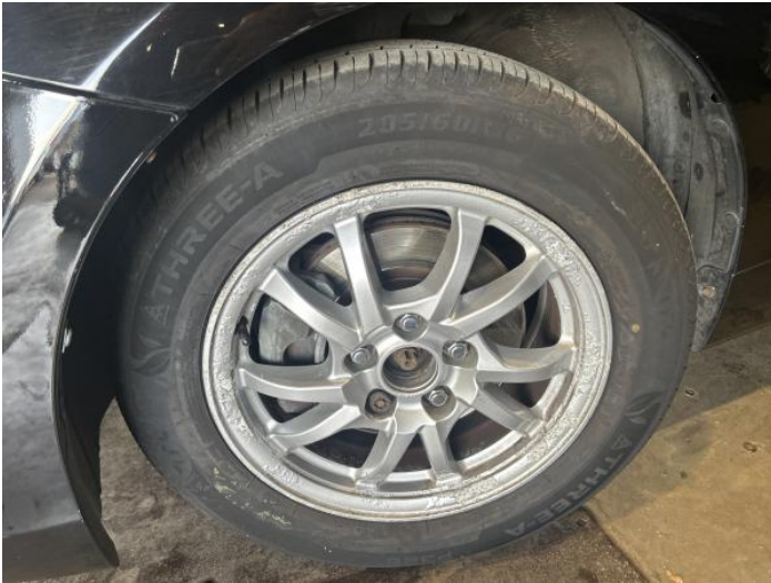
15: Wheel nsf Corroded Light
