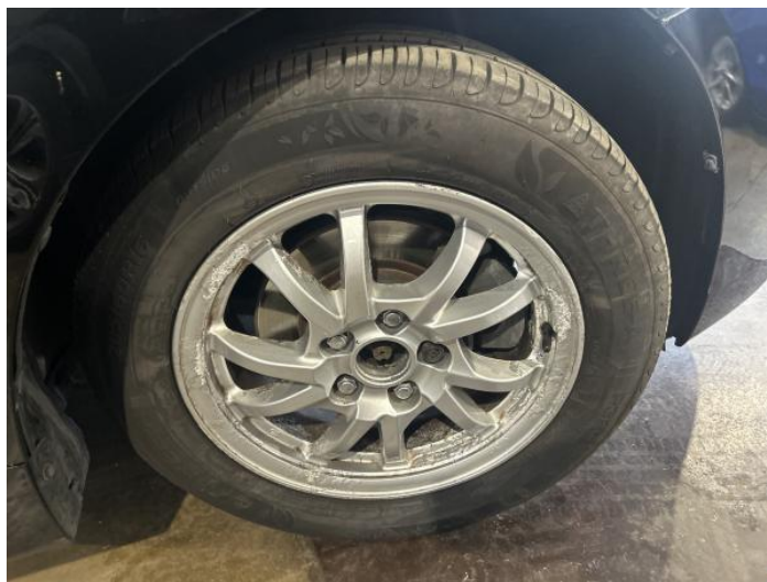
2: Wheel of Corroded Light
