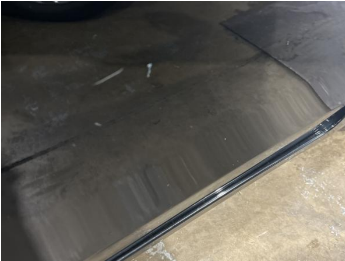
3: Door osf Scratched UpTo 25mm Thru Paint
