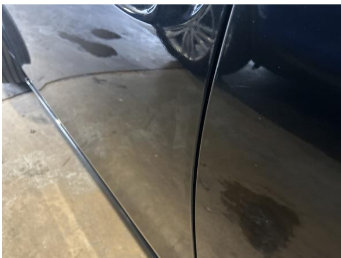
14: Door nsf Dented Over 30mm
