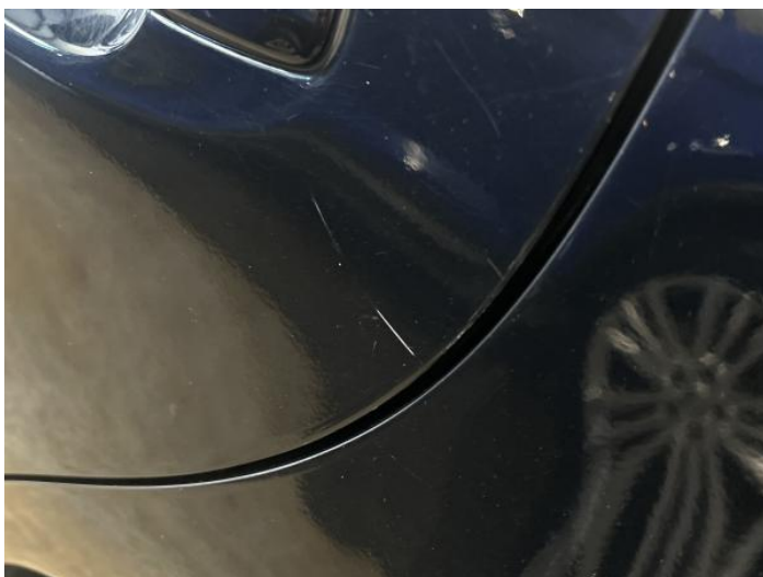
12: Door nsr Scratched UpTo 25mm Thru Paint
