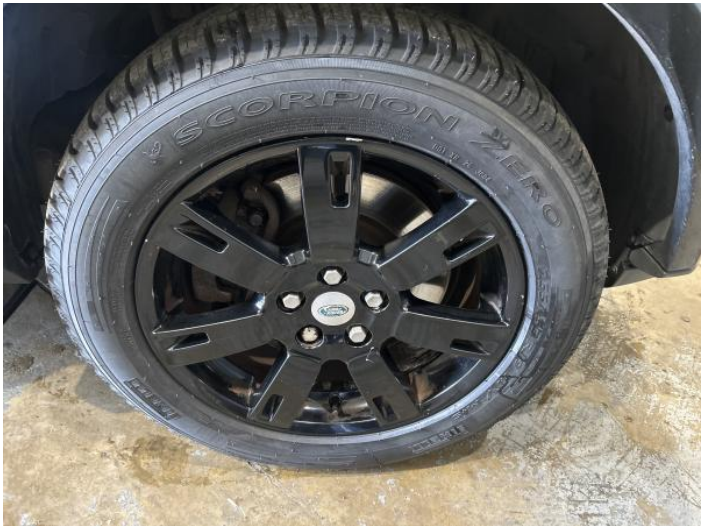
2: Wheel osf Scratched Up To 50mm
