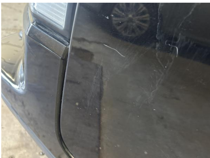
7: Qtr Panel osr Scratched UpTo 25mm Thru Paint
