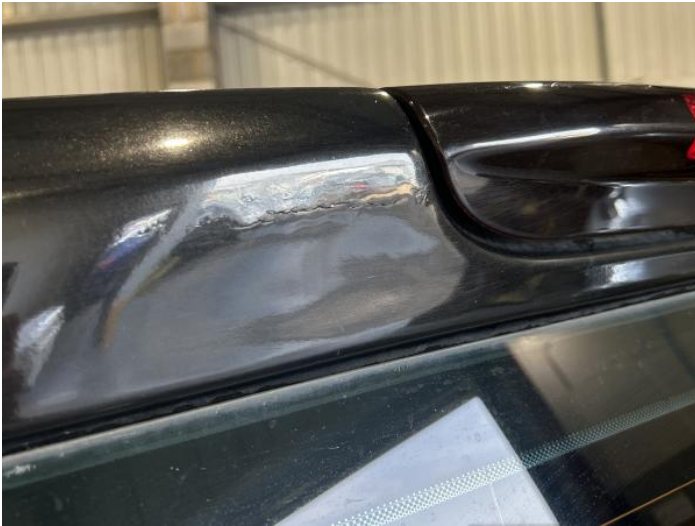
9: Boot Lid Poor Previous Repair Poor Paint
