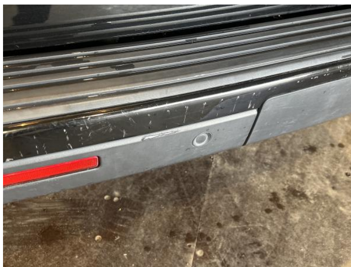
8: Bumper Rear Scratched Over 100mm Thru Paint
