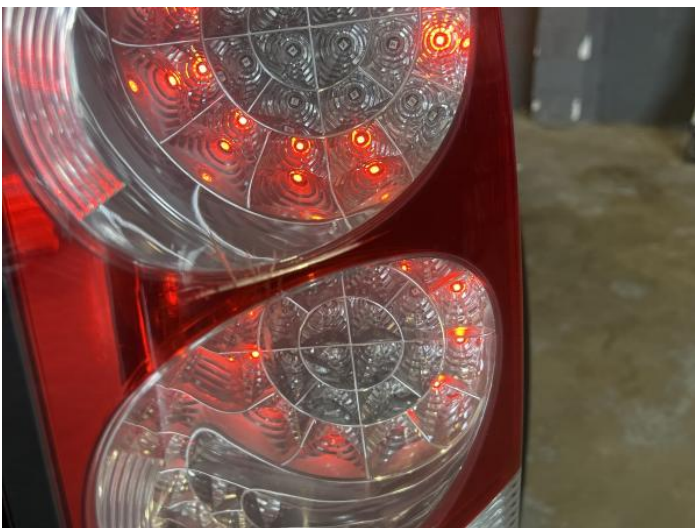
19: Lamp osr Broken Replace
