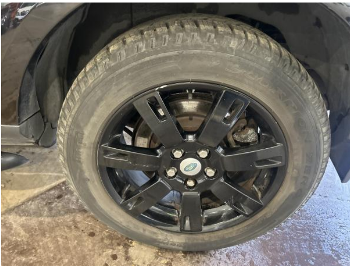
11: Wheel nsr Scratched Up To 50mm
