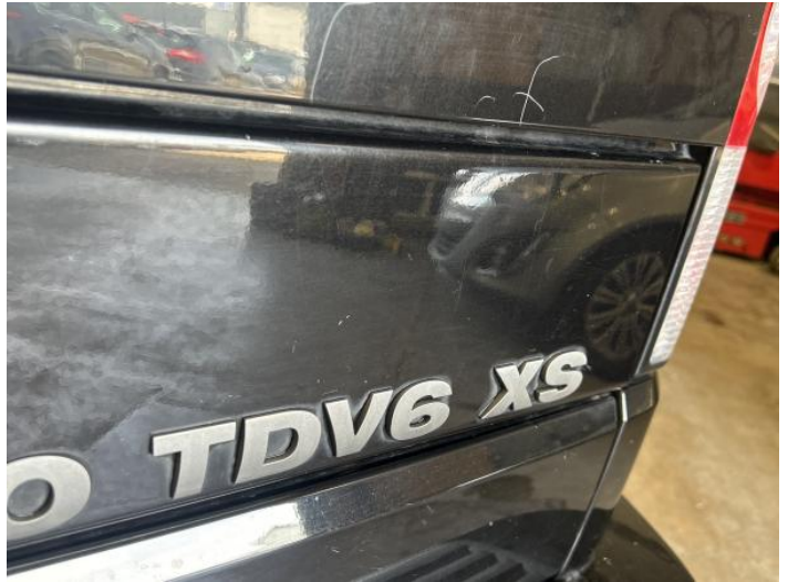
10: Tailgate Scratched Over 25mm Thru Paint
