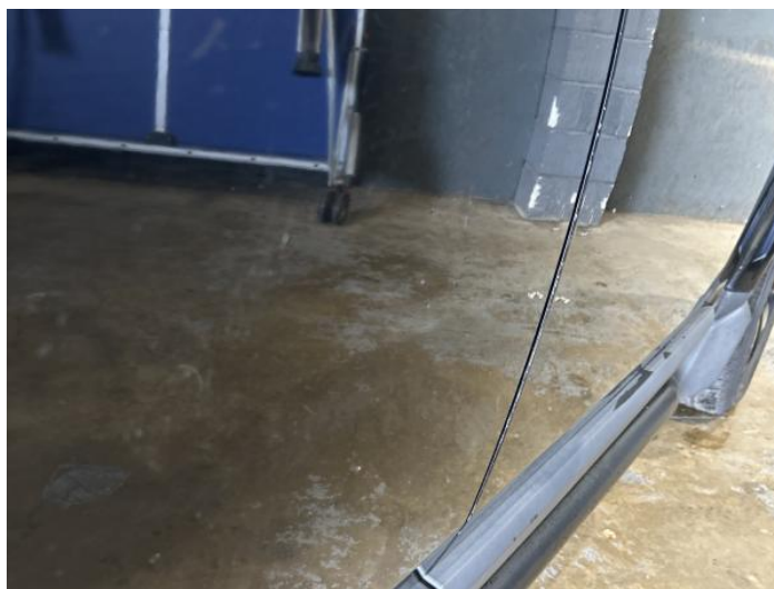
6: Door osr Dented Over 30mm
