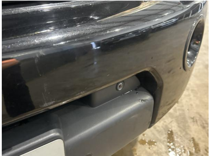
16: Bumper Front Scratched Over 100mm Thru Paint
