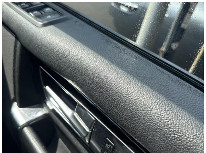
20: Door Pad osf Scuffed Over 25mm
