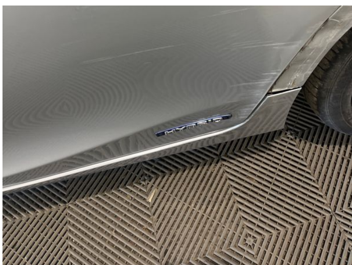
7: Door nsr Scratched Over 25mm Thru Paint
