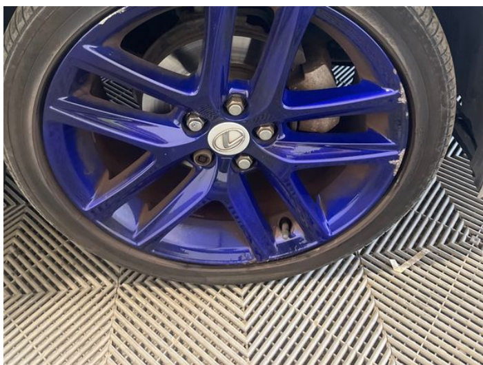
1: Wheel osf Scratched Over 50mm
