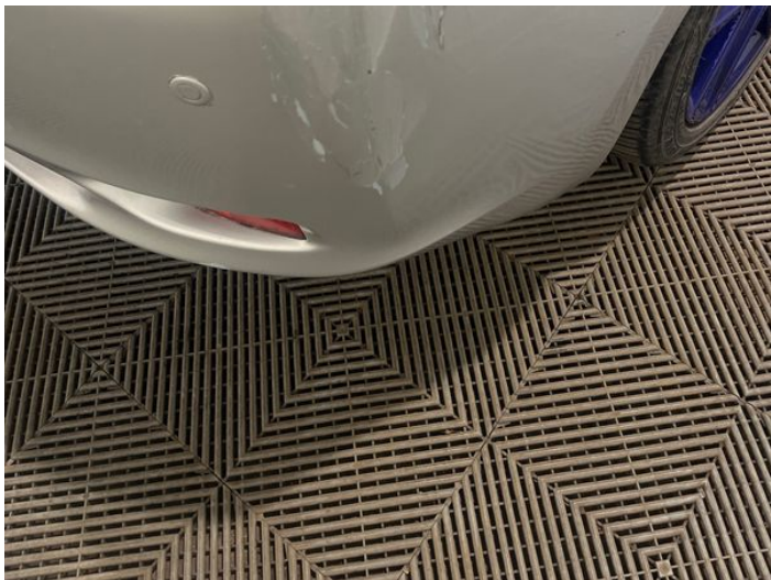
9: Bumper Rear Poor Previous Repair Paint Flake
