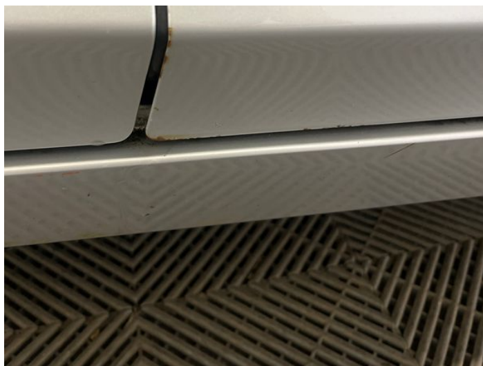
12: Door osf Rusted UpTo 5mm
