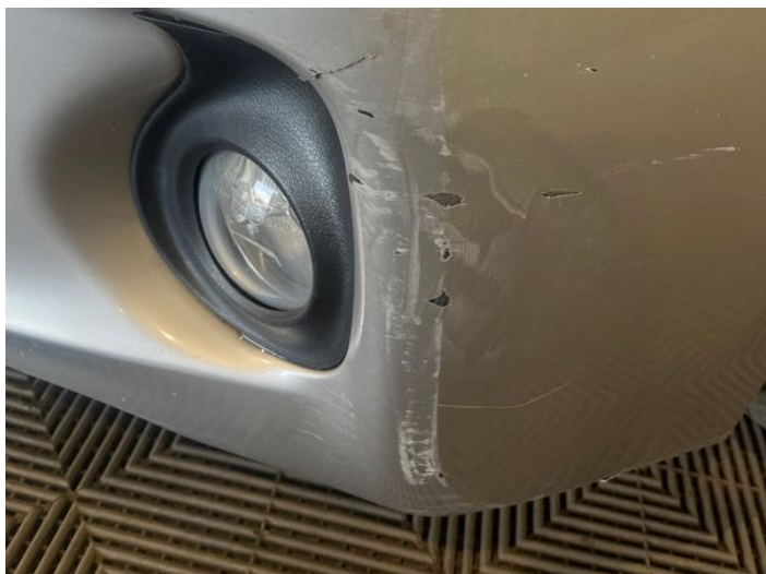
3: Bumper Front Cracked Over 25mm
