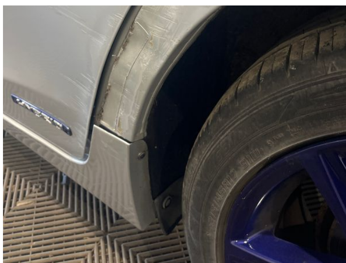
8: Qtr Panel nsr Dented With Paint Damage
