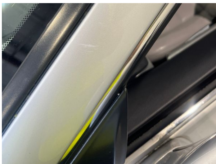
6: A Post ns Scratched UpTo 25mm Thru Paint
