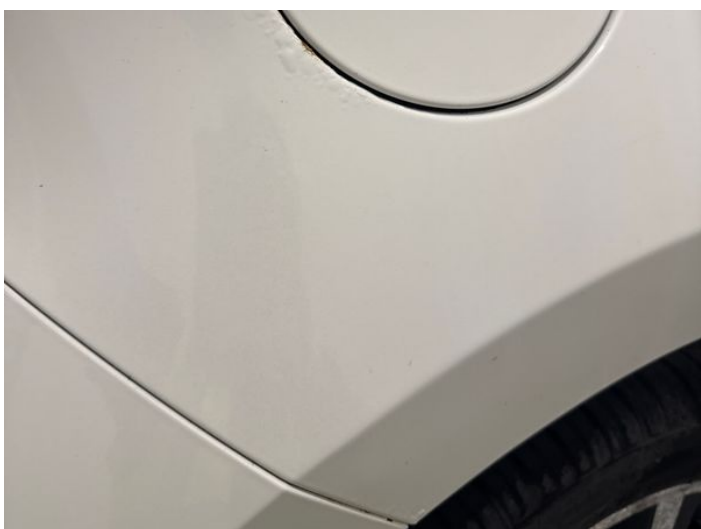
11: Qtr Panel osr Rusted Over 5mm
