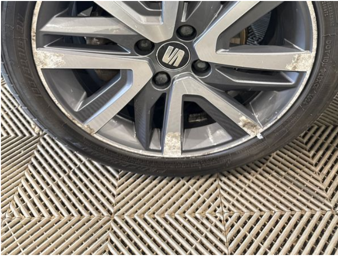
3: Wheel nsf Scratched Over 50mm
