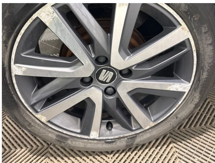
12: Wheel osr Scratched Over 50mm
