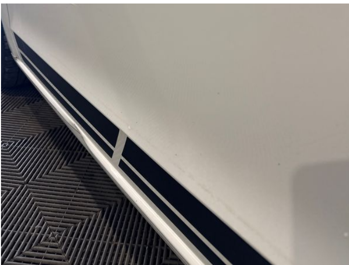
7: Door nsf Dented Between 10mm + 30mm
