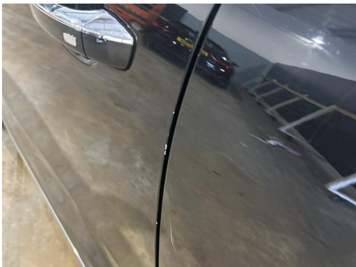
9: Door nsf Chipped Edge Chip
