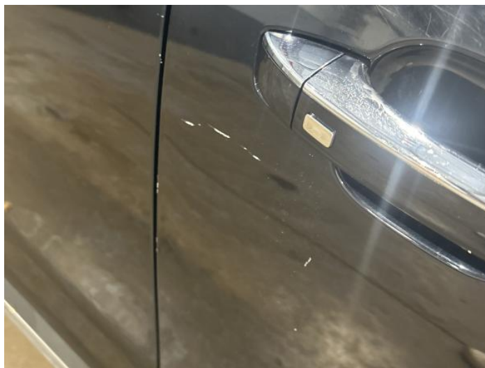
2: Door osf Scratched Over 25mm Thru Paint
