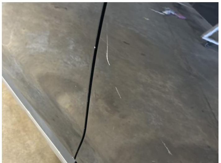
8: Door nsr Scratched Over 25mm Thru Paint
