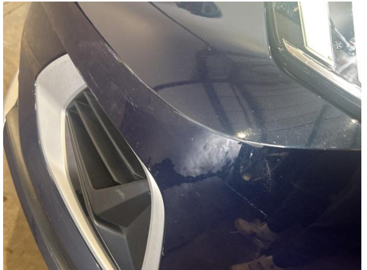
6: Bumper Front Scratched 25 to 100mm Thru Paint
