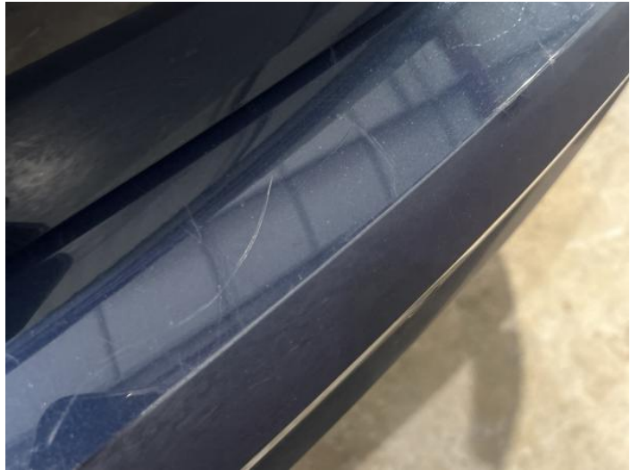
4: Bumper Rear Scratched Over 100mm Thru Paint
