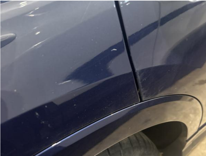
3: Qtr Panel osr Chipped 1 To 5
