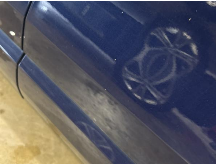
5: Door nsr Chipped 1 To 5
