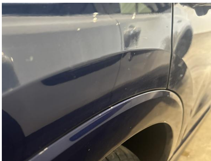
2: Qtr Panel osr Dented 2 Or Less UpTo 10mm
