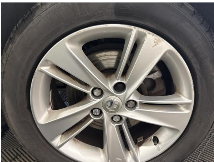
18: Wheel osf Scratched Over 50mm
