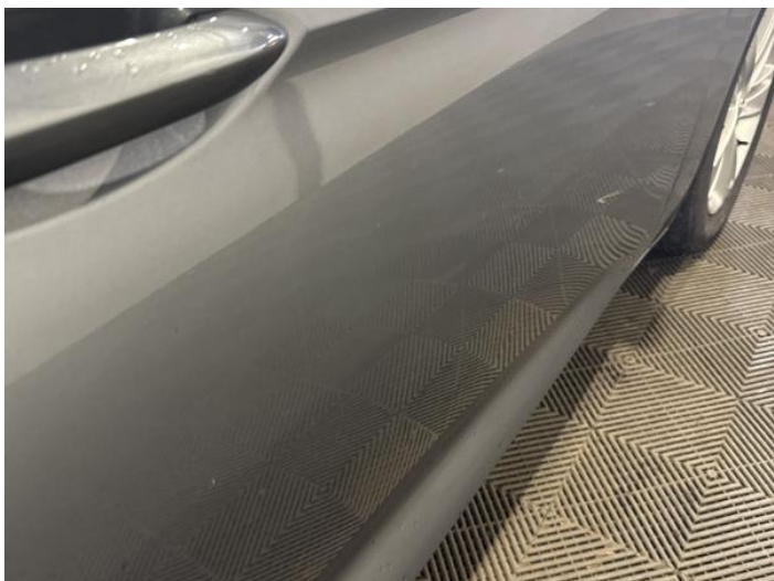
15: Door osf Scratched Over 25mm Thru Paint
