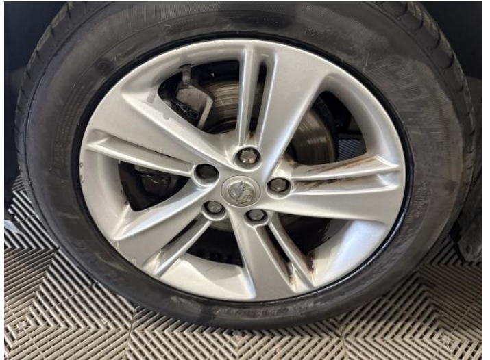
4: Wheel nsf Scratched Over 50mm
