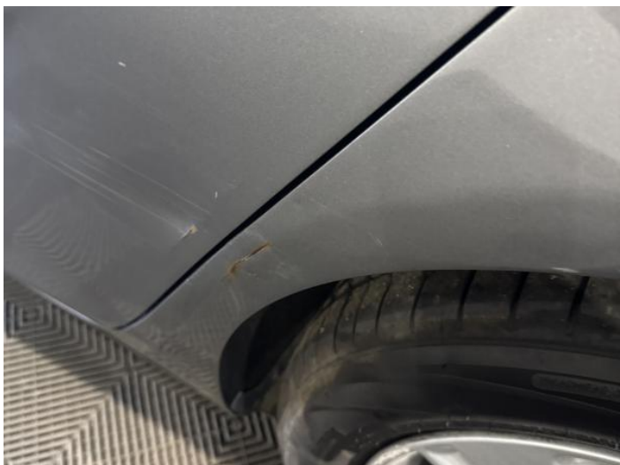
9: Qtr Panel nsr Cracked Replace
