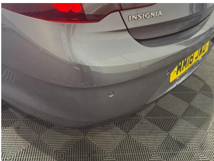
11: Bumper Rear Scratched Over 100mm Thru Paint
