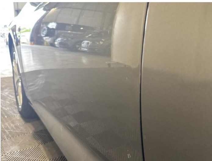
7: Door nsf Poor Previous Repair Rippled UpTo 30%
