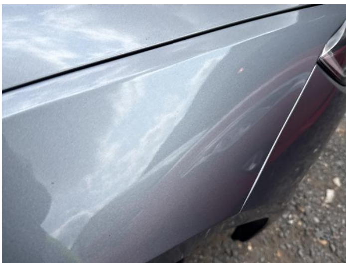
20: Wing osf Dented Between 10mm + 30mm
