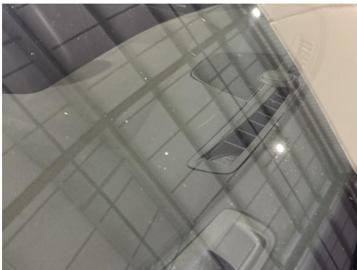
16: Screen Front Chipped UpTo 10mm
