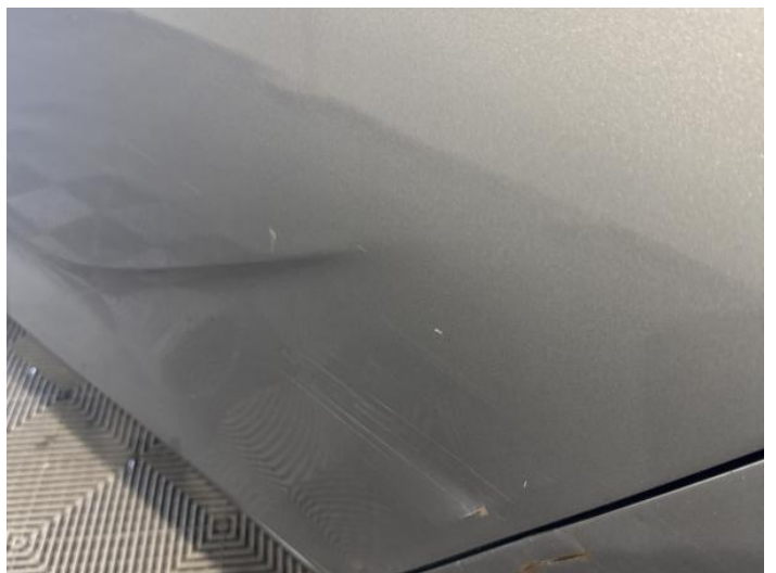
8: Door nsr Dented With Paint Damage
