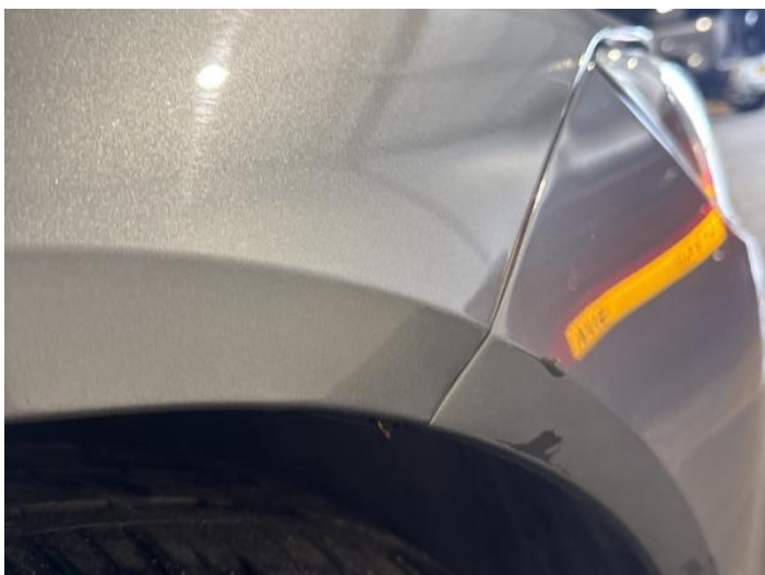
17: Wing osf Scratched UpTo 25mm Thru Paint
