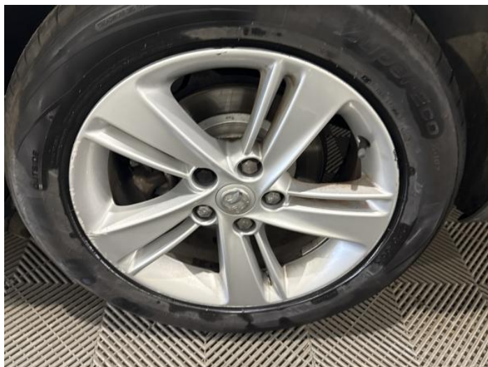
10: Wheel nsr Scratched Over 50mm
