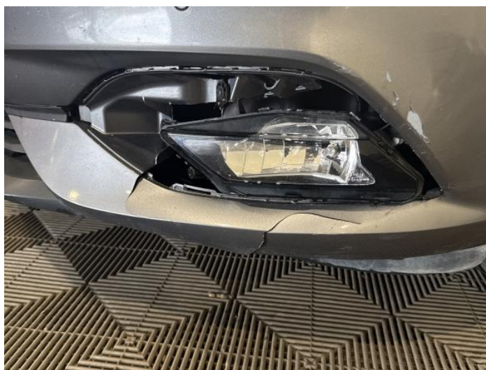
2: Fog Lamp Surrounds Missing Replace
