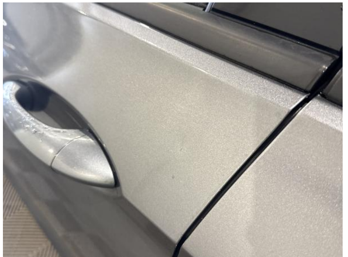
6: Door nsf Dented Between 10mm + 30mm
