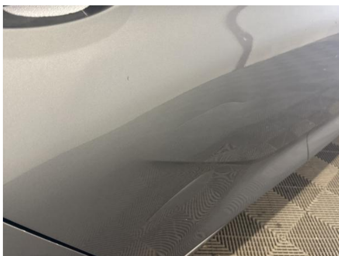
14: Door nsr Dented With Paint Damage
