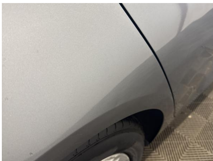
12: Qtr Panel osr Dented Between 10mm + 30mm
