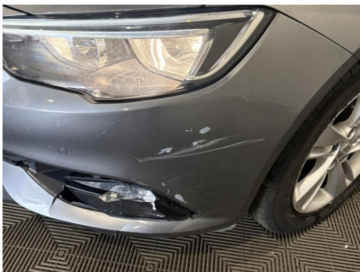
1: Bumper Front Cracked Over 25mm
